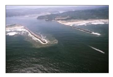
were completed in 1979 at a cost of \$1.9 million. Local interests requested the boat basin entrance channel be deepened to 15 feet and extended to serve a new moorage area. Deepening of the Charleston channel and turning basin was completed in 1985 under Section 107 of the Rivers and Harbors Act of 1960. The total federal cost was \$1.2 million.
