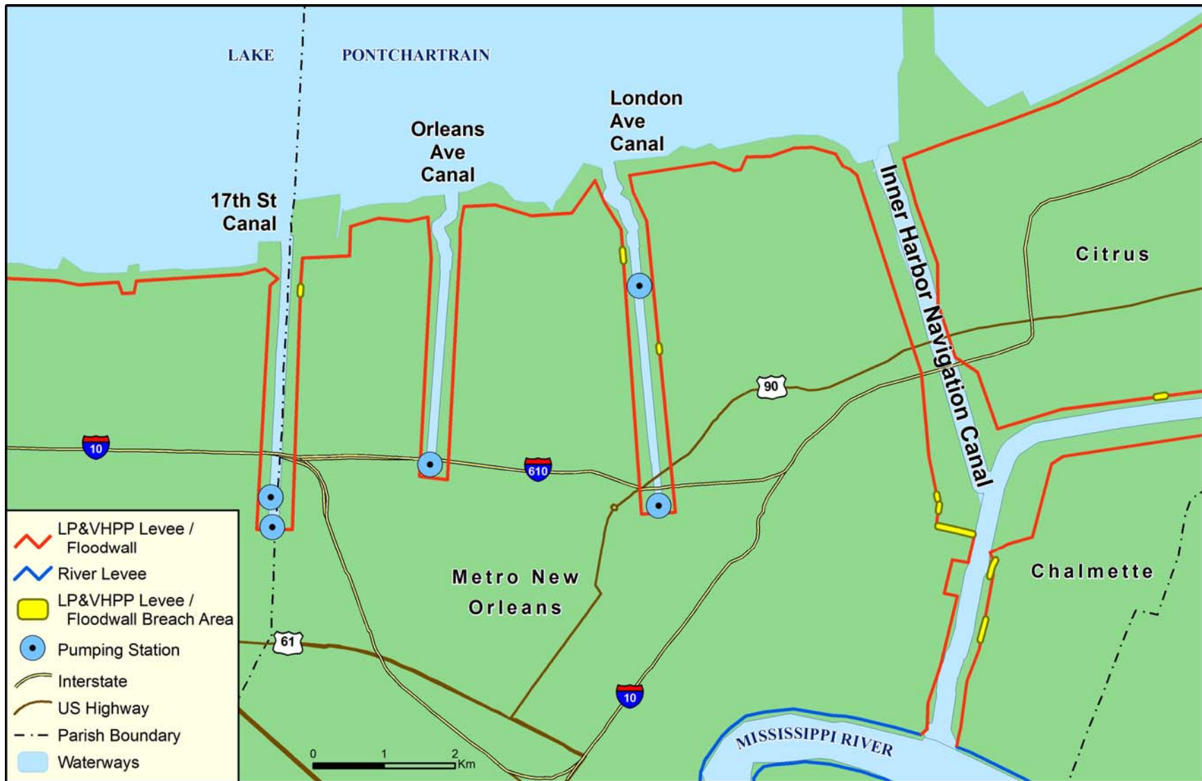
Map 4-1: LP&VHPP Structures and Breach Areas on the Outfall Canals and the Inner Harbor Navigation Canal
