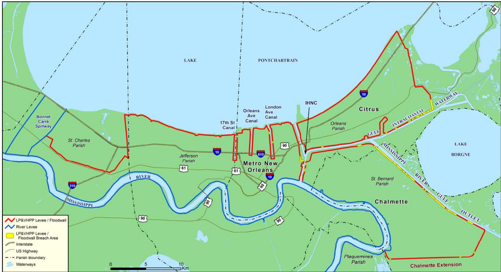
Map 2-1: The LP&VHPP Area, Protective Structures, and Breach Areas
