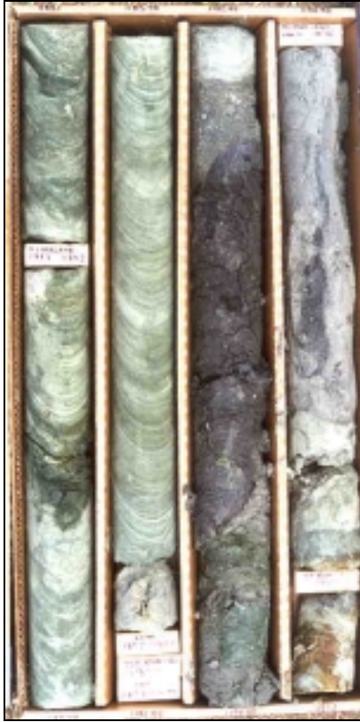
Figure 4. Cores of crater unit B from depth of about 1,185 feet. Note the high-angle bedding at left and the possible fluidization feature at the far right. Top of core is at upper left. Nominal core diameter is 2.4 inches.
