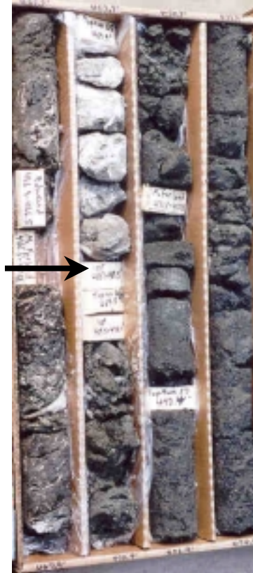
Figure 10. Contact at 470.9 ft (arrow) between fine-grained marine deposits of the Old Church Formation and overlying shelly and locally cemented sediments of the Newport News beds of the Calvert Formation. Top of core is at upper left. Nominal core diameter is 2.4 inches.
