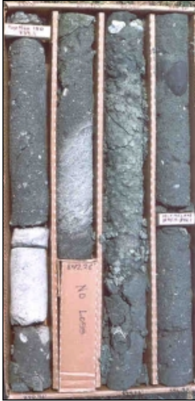
Figure 5. Cores of crater unit C from depth of about 830 feet. Limestone, glauconitic sand, and clay clasts “float” in a dark-gray, muddy, quartz-glaucanite sand matrix. Top of core is at upper left. Nominal core diameter is 2.4 inches.
