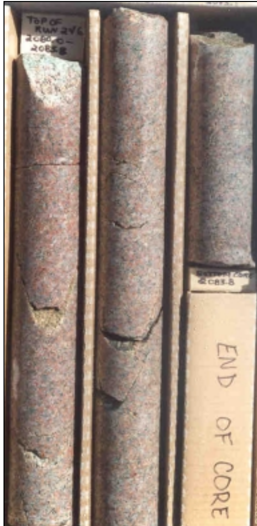
Figure 2. Granodiorite from the bottom of the Langley core. Top of illustrated core is at upper left. Nominal core diameter is 2.4 inches.
