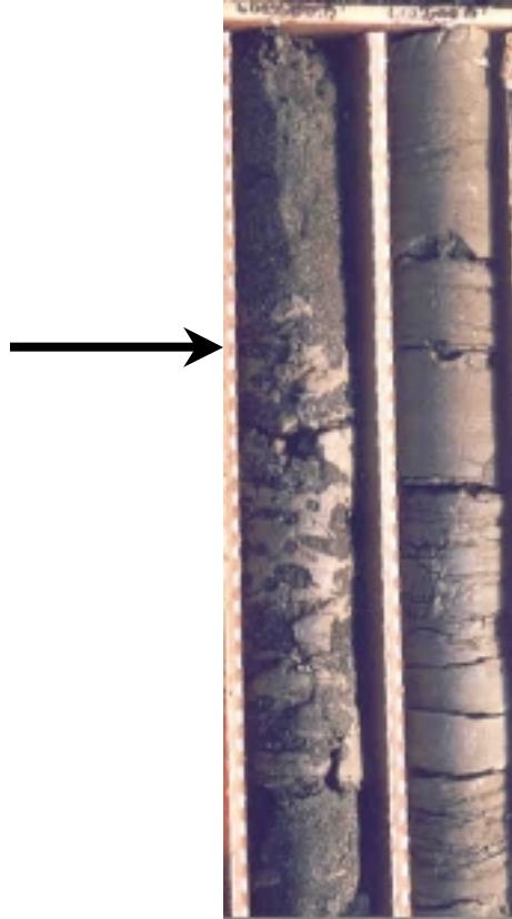
Figure 8. Highly burrowed contact interval (tray at left) between fine-grained marine sediments of the Chickahominy Formation (at right) and quartz-glaucinite sand at the base of the overlying Delmarva beds. Arrow is at the formation contact (601.3 ft). Top of core is at upper left. Nominal core diameter is 2.4 inches.
