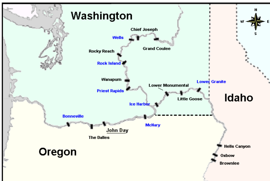
Figure 1. Location of hydroelectric projects of the Federal Columbia River Power System on the Columbia and Snake rivers. Facilities with adult PIT detection capabilities are in blue.
