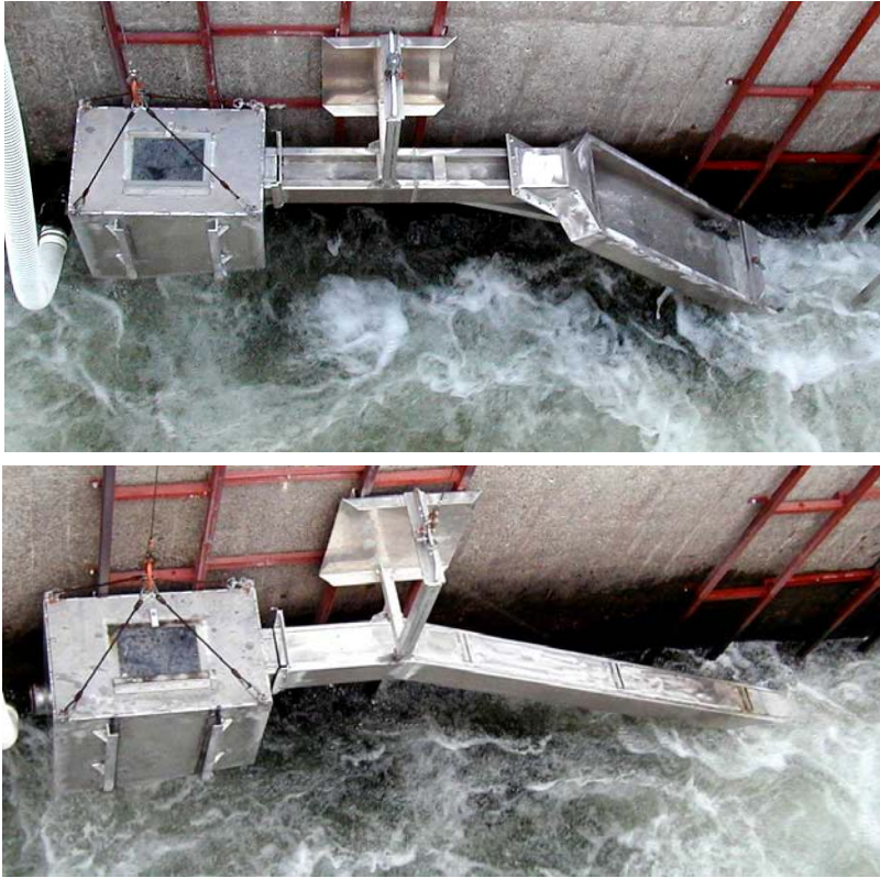
Figure 2. Prototype lamprey collectors tested in the Bradford Island AWS.
