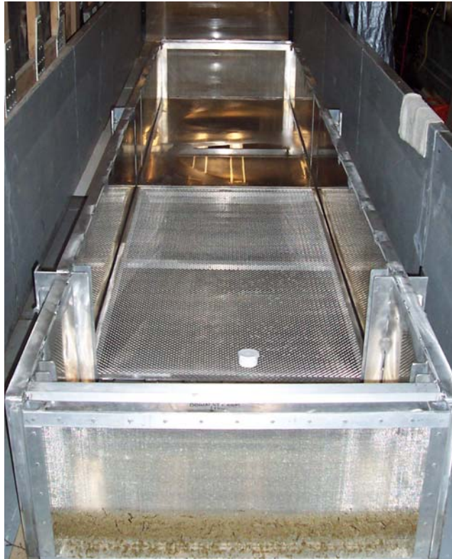
Figure 4. Flume insert within the main flume channel at McNary Dam.
