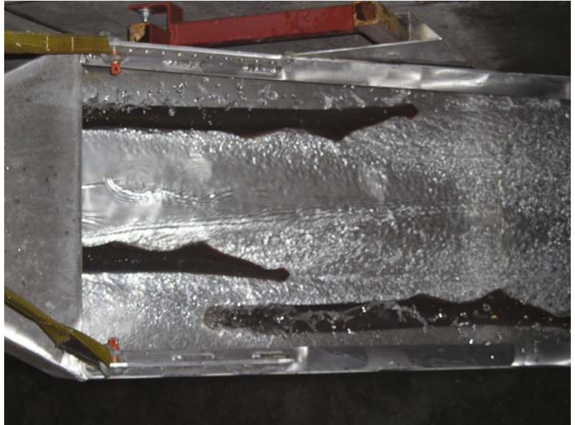
Figure 1. Lamprey ascending a lamprey-specific passage structure (LPS) at Bonneville Dam.
