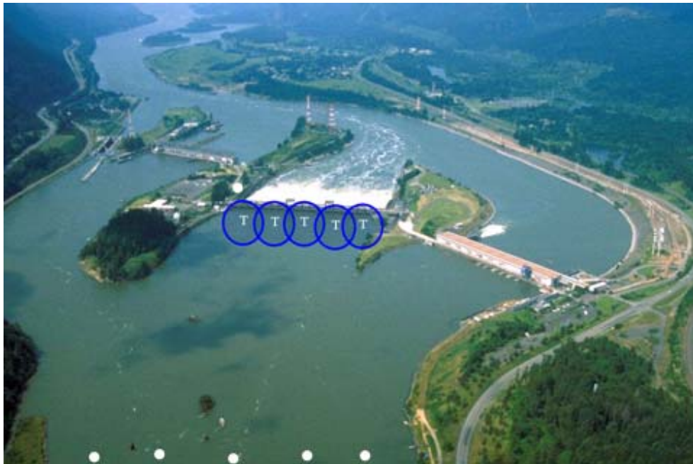
Figure 2. Photograph of Bonneville Dam Showing the Coverage of 2-D Tracking Nodes Mounted on Spillway Piers and Five Autonomous Nodes, Indicated by White Dots at the bottom, Forming a Project Entrance Array
