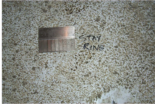
Figure A - 35. Bonneville Unit 4 stay ring top and bottom Ra @ 1100 – 1180 \mu inches
