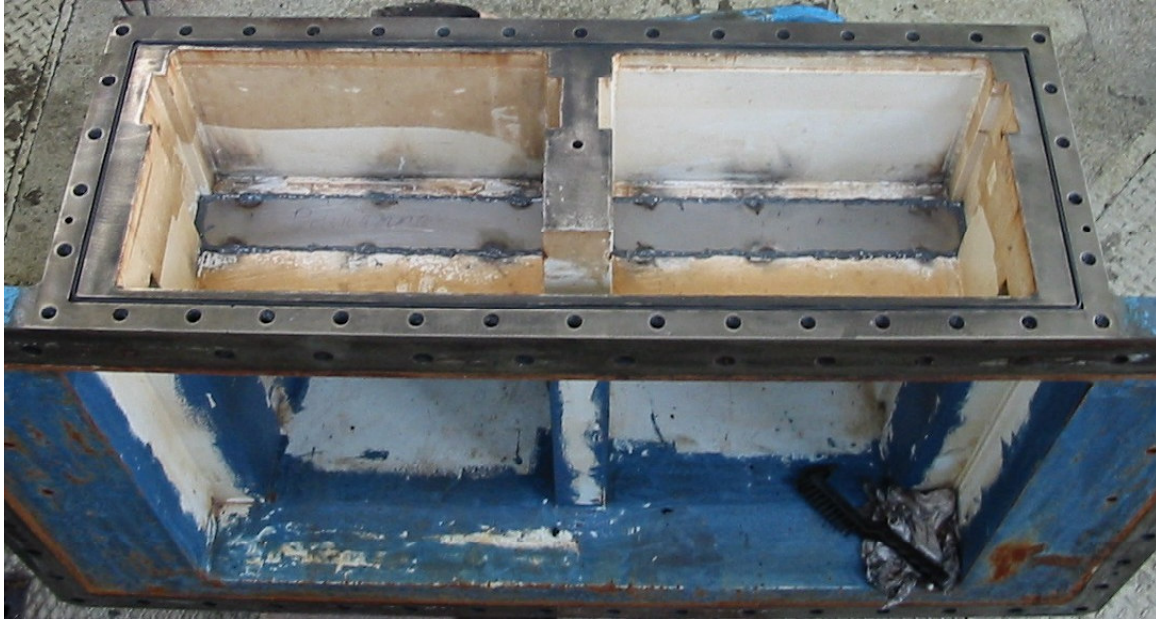
Figure A - 41. View of simplified stop log closure in a Snake River model
