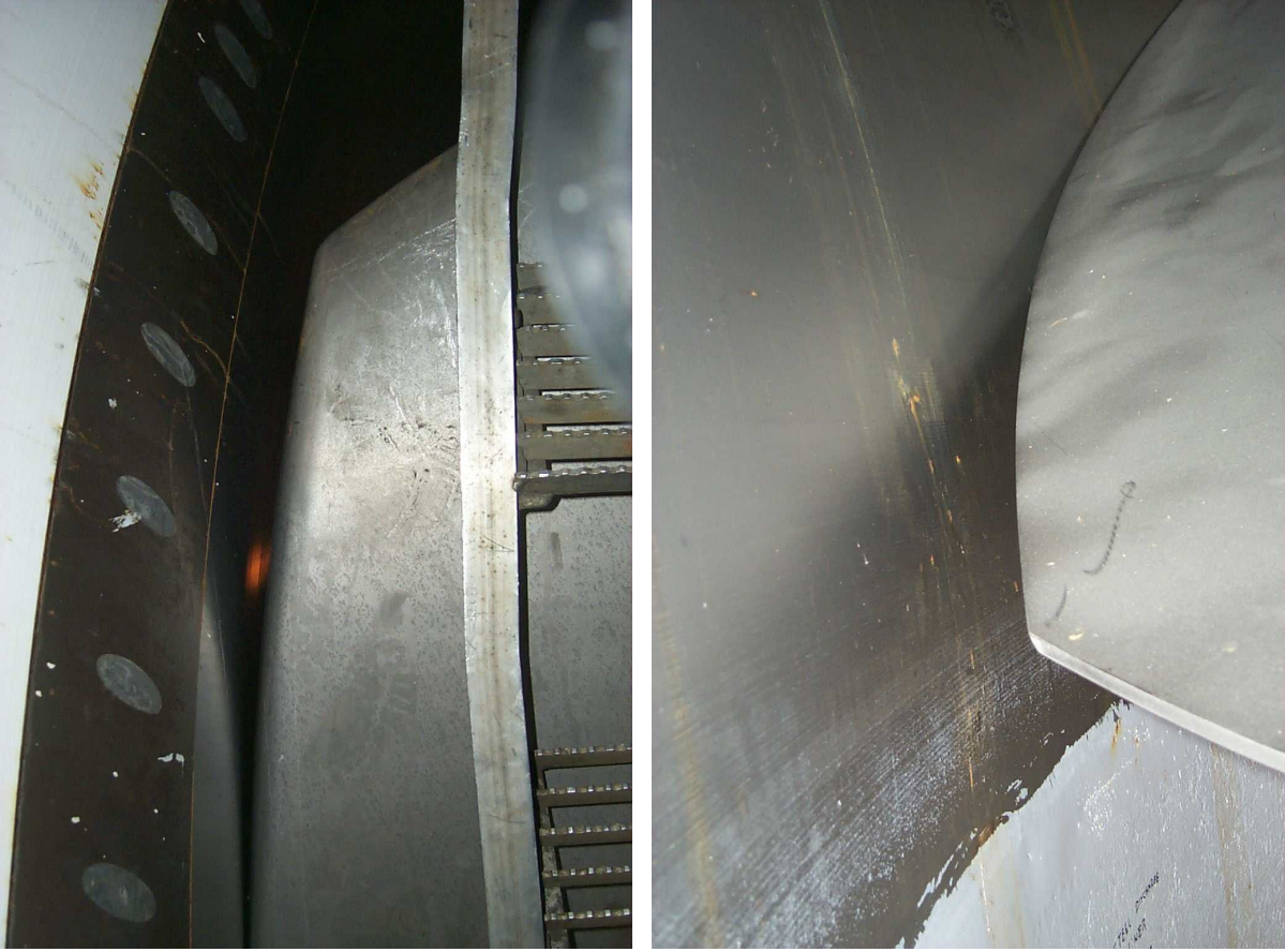
Figure 46. Leading edge gap at the maximum blade angle. Figure 47. Trailing edge gap at the maximum blade angle.
