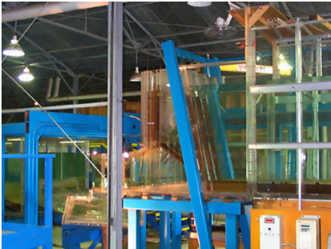
Figure 8. ERDC-WES McNary model with model runner and control instrumentation.
