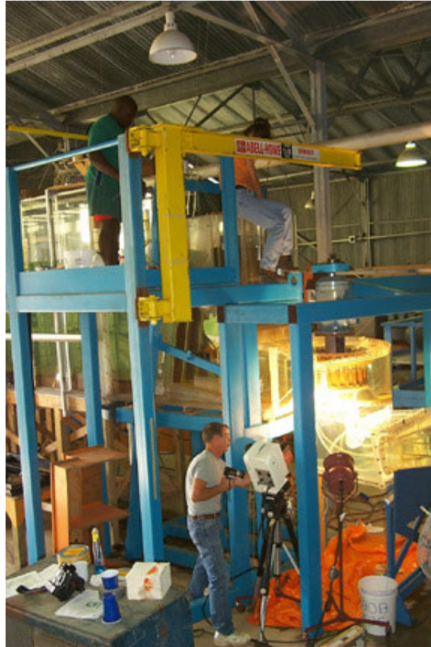
Figure 4. Setup of high-speed film cameras.
