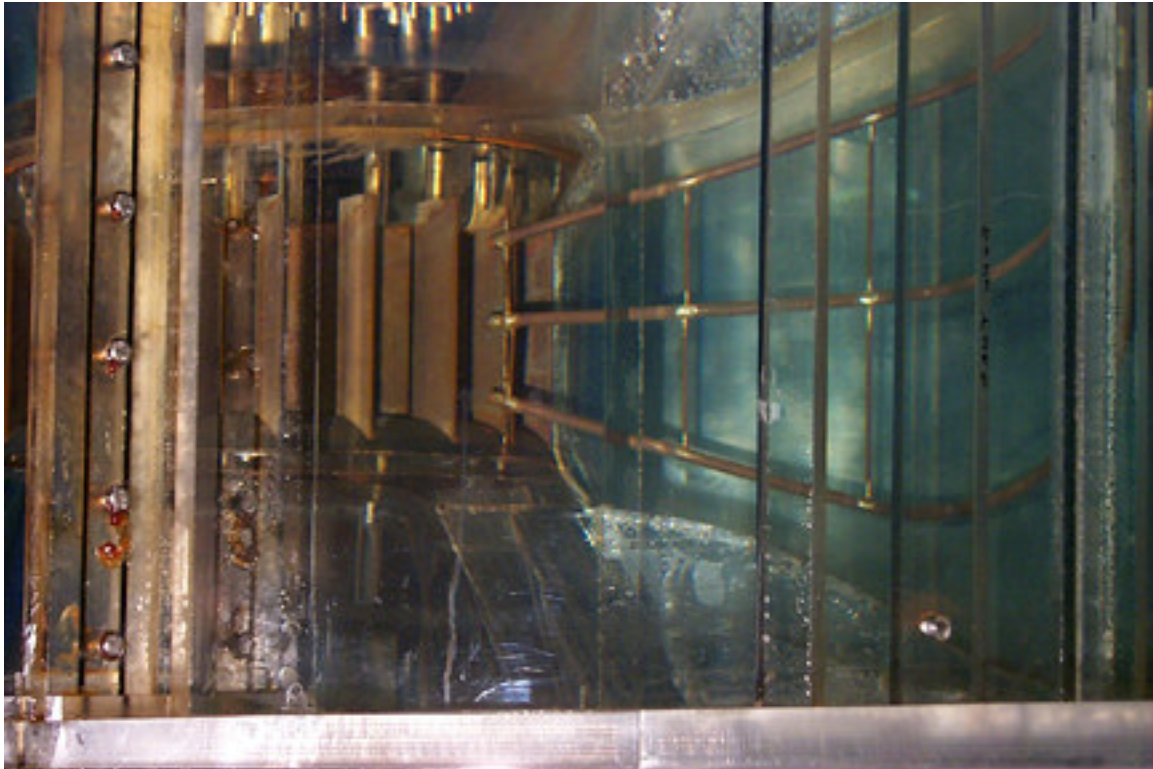
Figure 42. Bead release tubes used in the Bonneville model.
