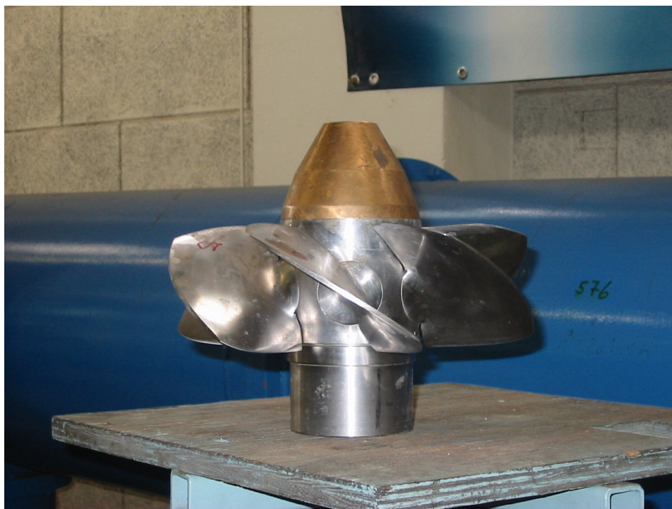
Figure 25. Existing Lower Granite model turbine runner.
