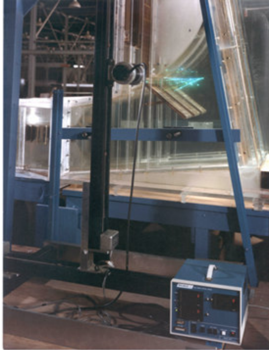
Figure 3. Laser Doppler velocity system.
