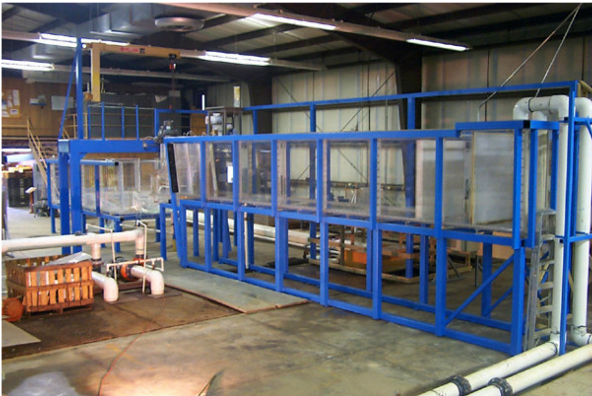
Figure 37. General view of new Bonneville 1:25-scale model.
