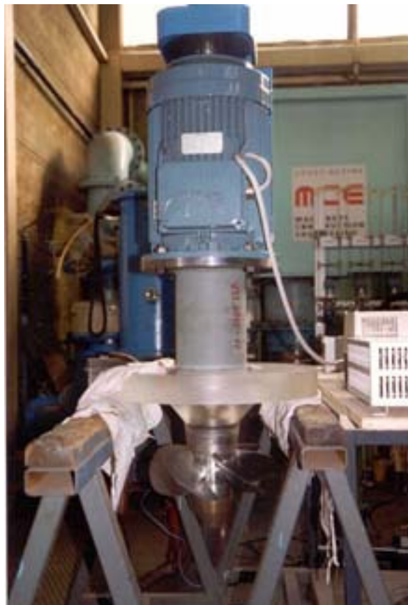
Figure 23. Lower Granite model turbine runner assembly and control instrumentation.
