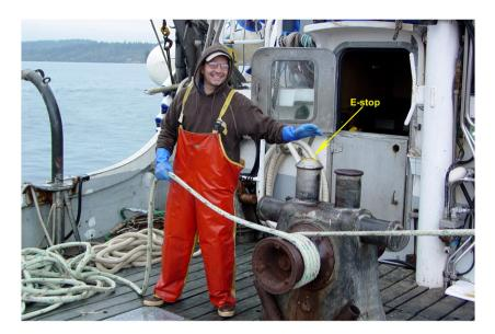
Fig. 3. Photo of Captain Bud Marrese with emergency-stop (e-stop) mounted on capstan-type winch.
