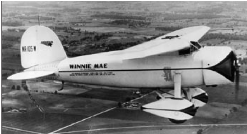
The Lockheed Vega of 1926 represented a dramatic departure from previous designs with its monocoque construction, NACA cowling, and teardrop wheel pants. Wiley Post flew the Lockheed Vega 5-B "Winnie Mae" solo around the world in only seven and one-half days during the summer of 1933. (SI Negative No. A-47516)
