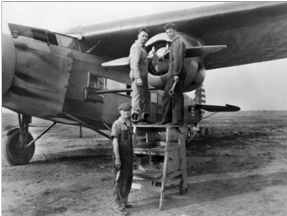
The NACA worked to improve existing designs such as the Fokker Trimotor with the addition of experimental low-drag cowlings and streamline engine nacelles in 1929. (NASA Image No. L-03333)
