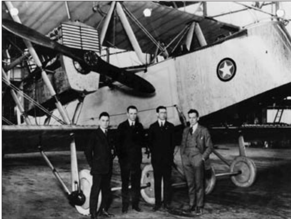
Aircraft such as the biplane, strut-and-wire braced Martin MB-1 Bomber represented the state of the art in aerodynamic design circa 1917. The designers of the aircraft, Laurence D. Bell (left), Glenn A. Martin (second from right), Donald W. Douglas (right), and James Kindlerberger (not pictured), would use the advances of the design revolution to create vastly different aircraft. (Martin test pilot, Thomas E. Springer, is second from left.) (SI Negative No. 43067)
