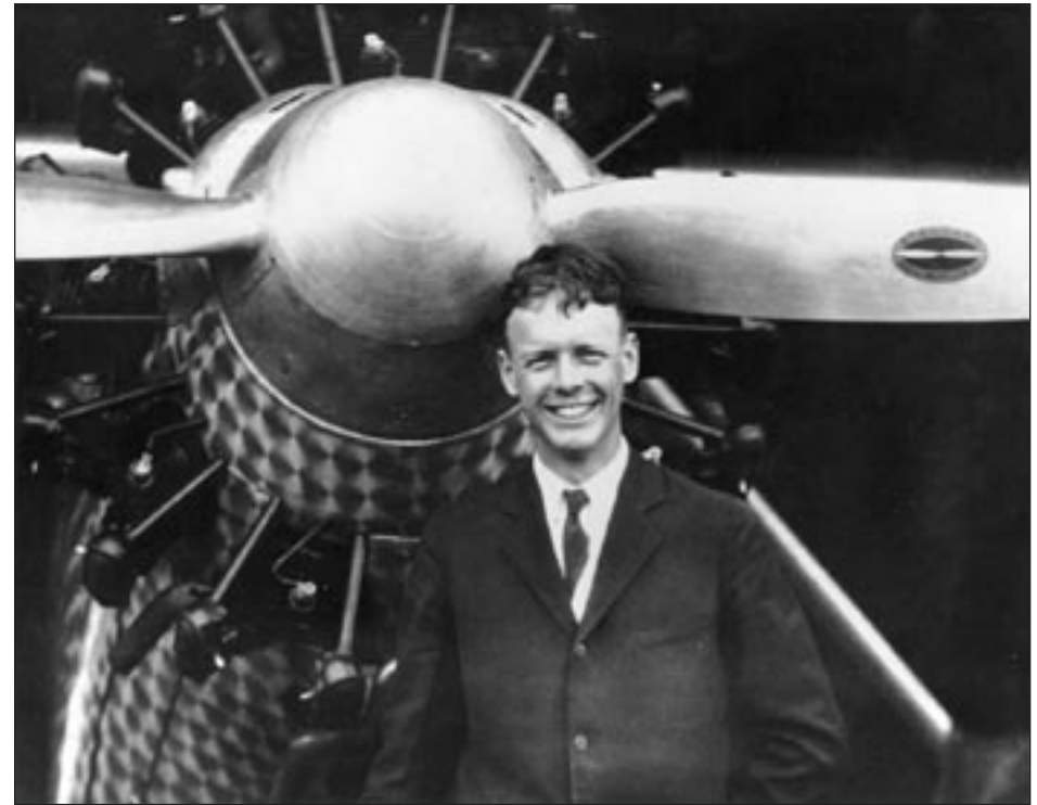
Lindbergh gambled that a ground-adjustable pitch propeller set just below the optimum setting for cruise would give him long-range efficiency while safely getting the Spirit of St. Louis off the ground at Roosevelt Field. The resultant dramatic takeoff for Paris on 20 May 1927 highlighted the need for variable-pitch propellers. (SI Negative No. A-4819A)
