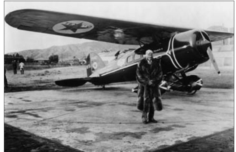
The inclusion of the NACA low-drag cowling to the Texaco Lockheed Air Express allowed Frank Hawks to establish a new Los Angeles to New York nonstop record of 18 hours, 13 minutes in February 1929. (SI Negative No. A31250-G; Videodisc No. 2B-11966)
