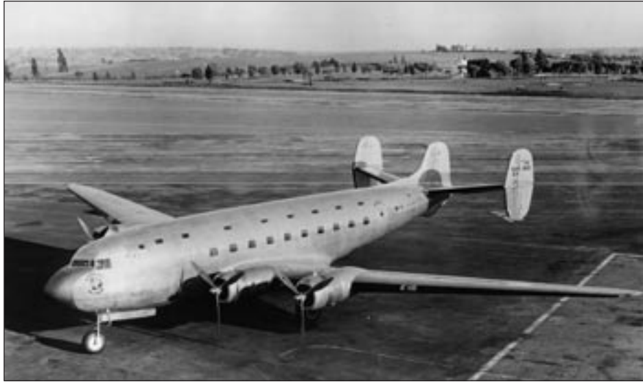
The one-and-only Douglas DC-4E represented many of the aerodynamic innovations that evolved during the 1920s and 1930s. It was the first large transport to use tricycle gear and its design process helped originate NACA research in the establishment of stability and control specifications prepared to insure good flying qualities. (SI Negative No. A0193510)
