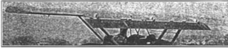
FIG. 3—Installation of Fowler wing with extension full out. Nose also
