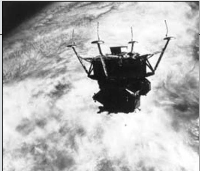
Apollo 9 Lunar Module in lunar landing configuration (AS09-21-3199)
