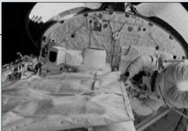
Astronaut Kathryn Sullivan checks the latch of the SIR-B antenna in Challenger's open cargo bay during STS-41G. The orbital refueling system (ORS) is just beyond the mission specialist's helmet. To the left is the large format camera (LFC). The LFC and ORS are stationed on a device called the mission peculiar experiment support structure (MPES). (STS41G-13-032)
