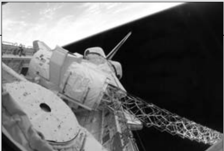
Part of the Shuttle Radar Topography Mission (SRTM) hardware is seen here through Endeavour's aft flight-deck windows about halfway through the scheduled 11-day SRTM flight on STS-99. The mast, only partially visible at lower right, is actually 60 meters (196.9 feet) in length. (S99-E-5476)
