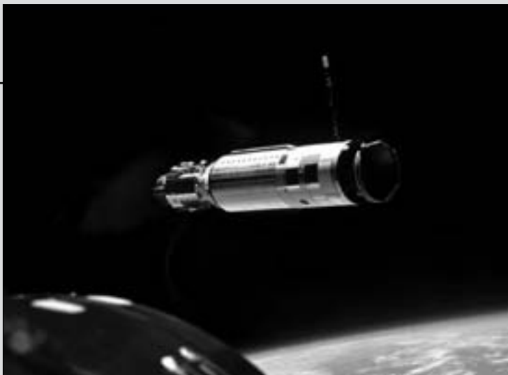
The Agena Target Vehicle as seen from the Gemini VIII spacecraft during rendezvous. (S66-25781)
