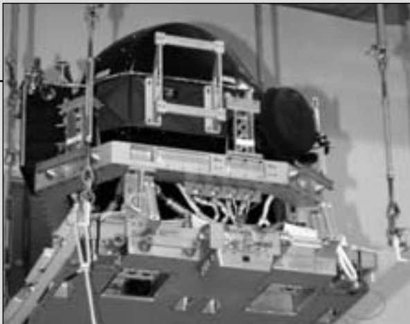
In the Space Station Processing Facility, the Control Moment Gyroscope (CMG), attached to the Small Adapter Plate Assembly, is lifted before being moved to the Lightweight Multi-Purpose Experiment Support Structure Carrier for flight. The CMG launched aboard Space Shuttle Discovery on Return to Flight mission STS-114. (KSC-05PD-0421)
