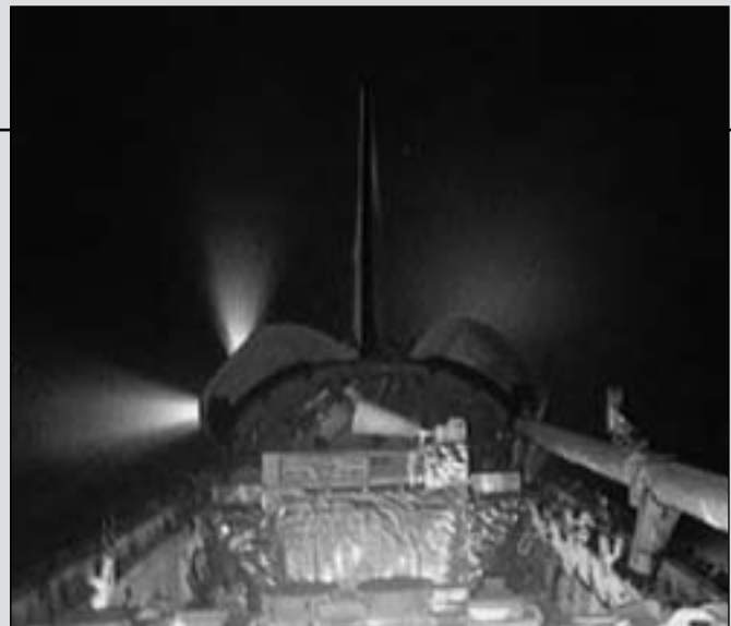
Discovery 's reaction control system jets fire during an on-orbit maneuver on STS-39. (STS039-27-016)
