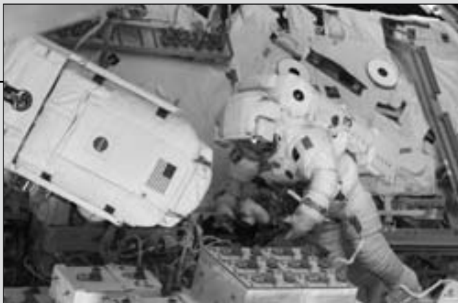
STS-111 mission specialists Franklin Chang-Diaz (left) and, representing the French Space Agency (CNES), Philippe Perrin (right) work on the Mobile Remote Servicer Base System (MBS) on the ISS. (MSFC-0201905)
