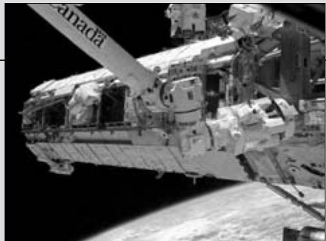
A view of the Starboard One (S1) truss, newly installed on the ISS, as photographed during the STS-112 mission's first scheduled session of extravehicular activity. (STS112-325-018)
