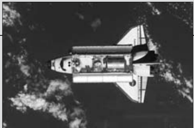
View of Space Shuttle Discovery as it approaches the ISS during the STS-105 mission. Visible in the payload bay of Discovery are the MPLM Leonardo, which stores various supplies and experiments to be transferred into the ISS, and the Integrated Cargo Carrier (ICC), which carries the Early Ammonia Servicer and two Materials International Space Station Experiment (MISSE) containers. (ISS002-E-9749)
