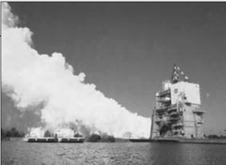
A cloud of extremely hot steam boils out of the flame deflector at the A-1 test stand during a test firing of a Space Shuttle Main Engine (SSME) at the John C. Stennis Space Center, Hancock County, Mississippi. (88-072-11)
