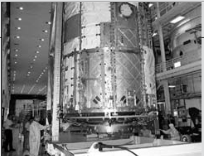
In the Operations and Checkout Building, the U.S. Lab named Destiny reaches the open floor after being lifted out of the vacuum chamber where it was tested for leaks. During STS-98, the crew installed the Lab on the Space Station during a series of three spacewalks in February of 2001. (KSC-00PP-0870)
