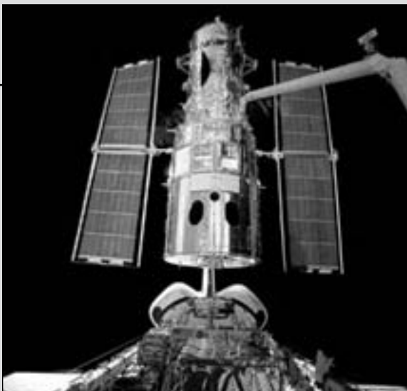
Attached to the Remote Manipulator System, the Hubble Space Telescope is unberthed and lifted up into the sunlight during STS-82, the second servicing mission. (STS082-709-097)
