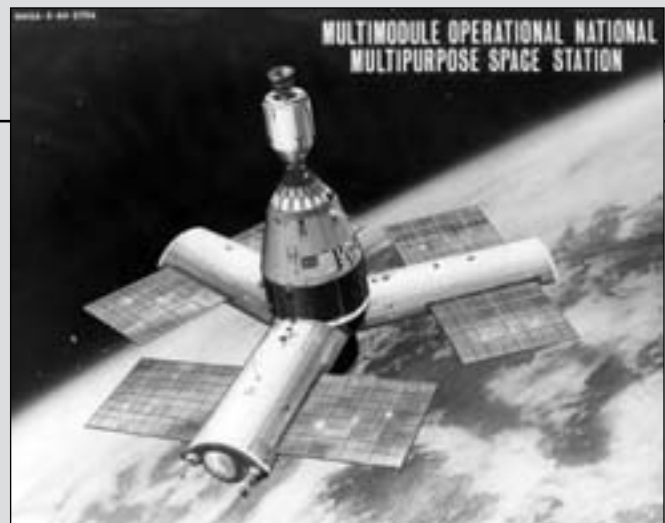
This three-radial-module space station concept was intended to utilize Apollo hardware to deploy the station and to transfer crews to and from orbit. (GPN-2003-00103)
