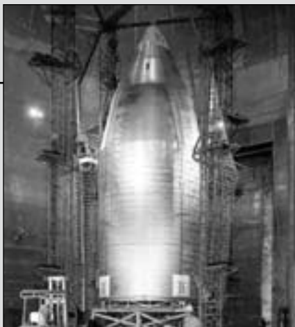
Skylab shroud installed in NASA Lewis Research Center’s (now known as Glenn Research Center) Plum Brook Station Space Power Facility. The shroud protected the upper section of the Skylab space station, including its solar power arrays. (GPN-2000-001462)
