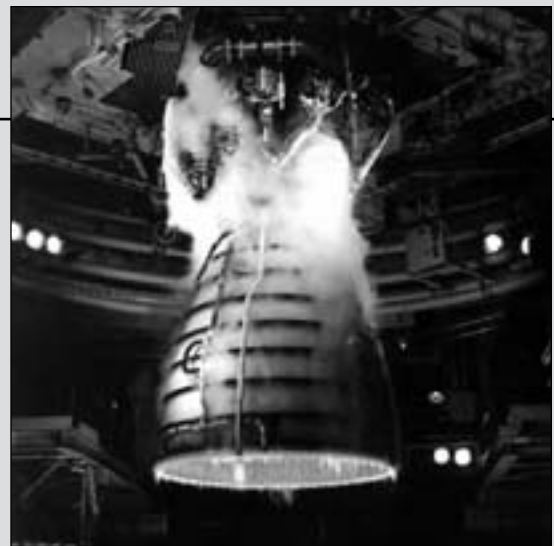
A remote camera captures a close-up view of a Space Shuttle Main Engine during a test firing at Stennis. (GPN-2000-000543)
