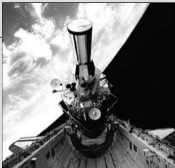
Defense Support Program (DSP)/Inertial Upper Stage spacecraft tilted to predeployment position in Atlantis 's payload bay on STS-44. (STS044-71-011)
