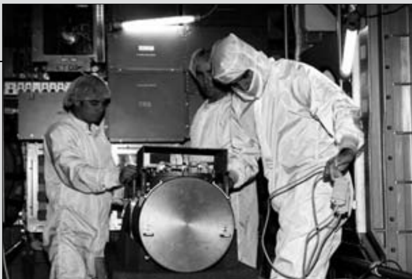
In the SPACEHAB Payload Processing Facility, McDonnell Douglas-SPACEHAB technicians prepare a Russian-made oxygen generator for flight in a SPACEHAB Double Module. The oxygen generator was delivered to Mir during STS-84. (KSC-97PC-0676)
