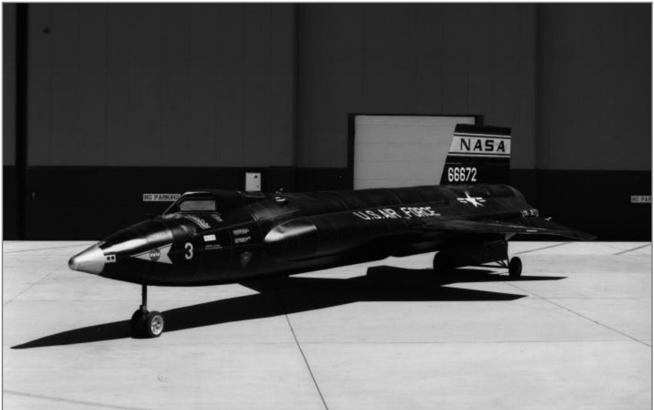
A refurbished mock-up of the famous X-15 aircraft was displayed at the Dryden Flight Research Center in 1995. The original three X-15 aircraft flew a combined total of 199 times from 1959 to 1968. These rocket-powered aircraft reached altitudes of more than 350,000 feet and speeds up to 4,520 miles per hour.
