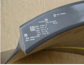
A Rolls-Royce T500 blade labeled with direct part marking technology
