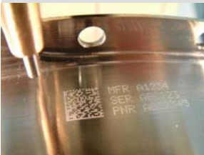
Dot-peen marking a 2D Data Matrix code onto an aero engine part
