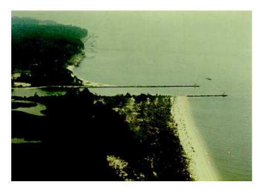
A stone jetty system was constructed at Herring Bay, St. Mary's County, Maryland, to stabilize the inlet and reduce shoaling of the channel. Interruption of the longshore transport of sand by the jetty system resulted in accretion of the updrift shoreline and erosion of the downdrift shoreline at Tall Timbers. To mitigate the erosion problem, the Corps constructed a stone revetment and placed approximately 250 linear feet of beachfill along a portion of the Tall Timbers shoreline.
