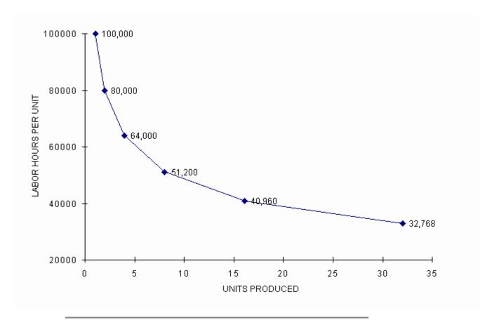
The graph is a curve because the number of hours of reduction between doubled quantities is constantly declining and an increasing number of units are required to double the quantity produced. Note that most of the improvement takes place during the early units of production. The curve will eventually become almost flat. The number of production hours could become quite small but it will never reach zero.
