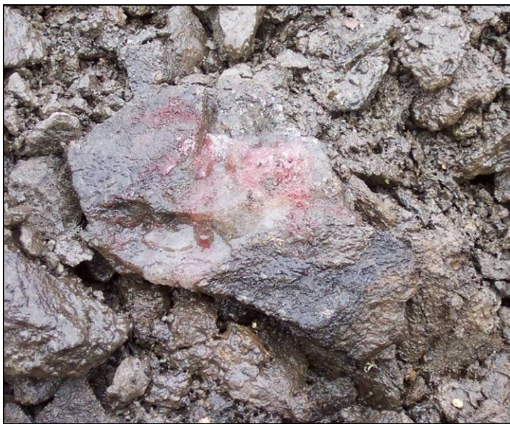
Figure 4-22. When alpha, alpha-dipyridyl dye is applied to a soil containing reduced iron, a positive reaction is indicated by a pink or red coloration to the treated area.
