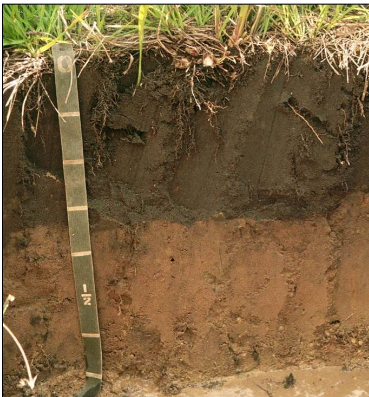
Figure 5-7. An anomalous bright sandy soil. This example has a relatively thick surface layer. Scale in 4-in. (10-cm) increments.
