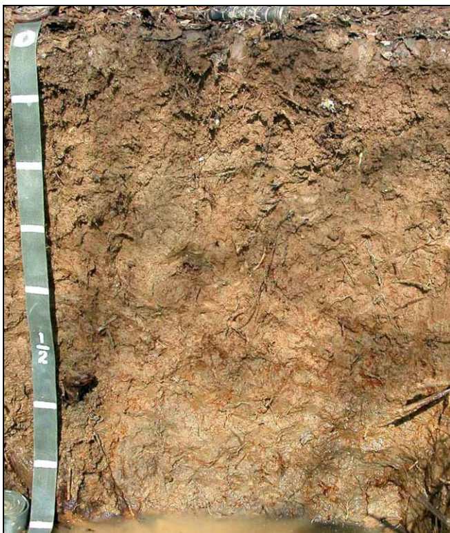
Figure 3-30. This indicator is restricted to floodplains that are actively receiving sediments. Photo by M. Rabenhorst. Scale in 4-in. (10-cm) increments.
