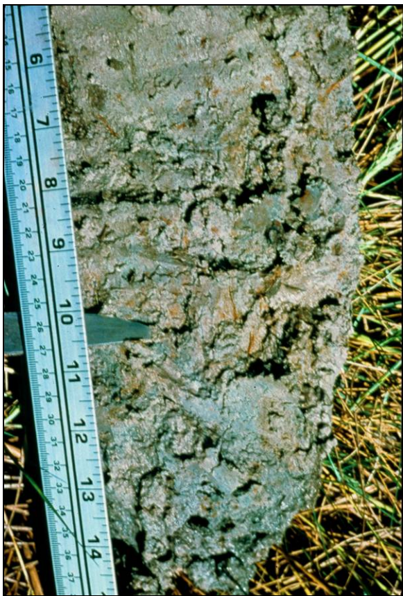
Figure 3-19. Indicator F3, Depleted Matrix. Redox concentrations are present within a low-chroma matrix.
