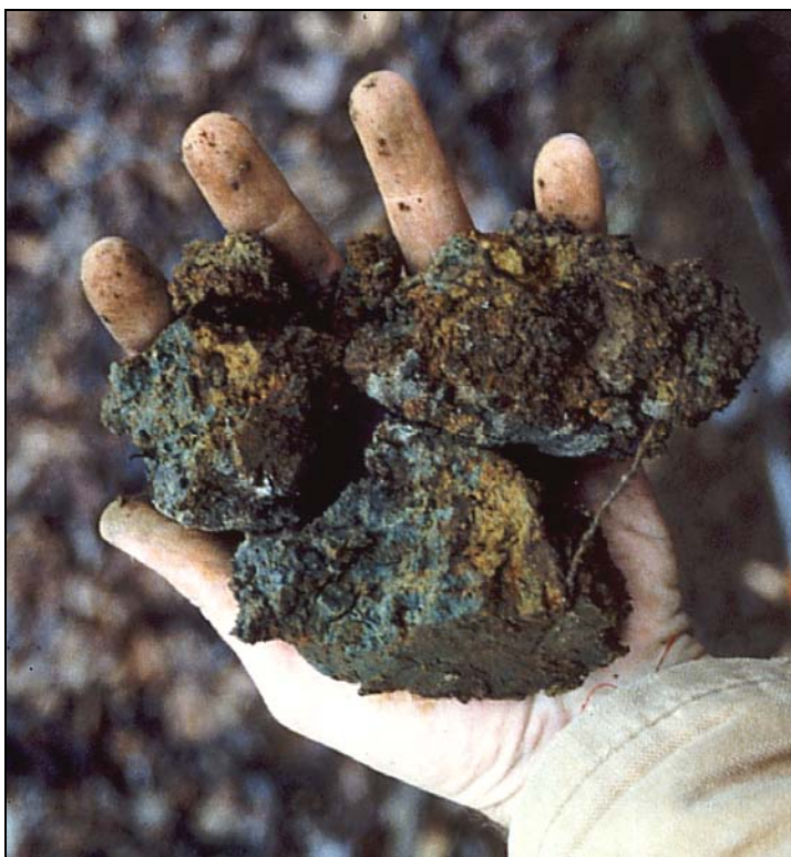
Figure 5-4. Non-hydric soils that are high in glauconite can have colors similar to hydric soils. In hydric soils, glauconite can mask redoximorphic features.
