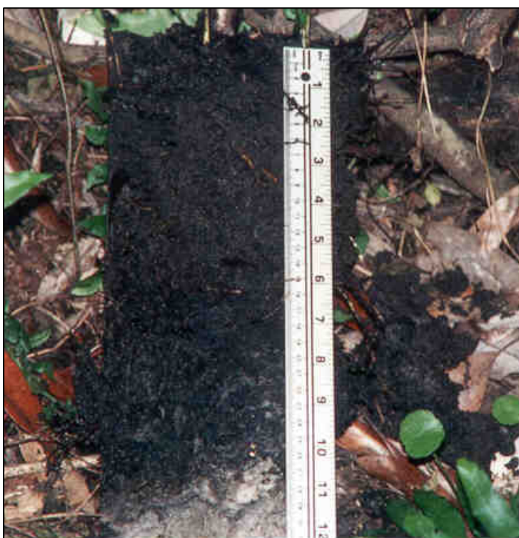
Figure 3-7. The mucky mineral layer in this example is about 4 in. (10 cm) thick and begins at the soil surface. Scale in inches (right) and cm (left).
