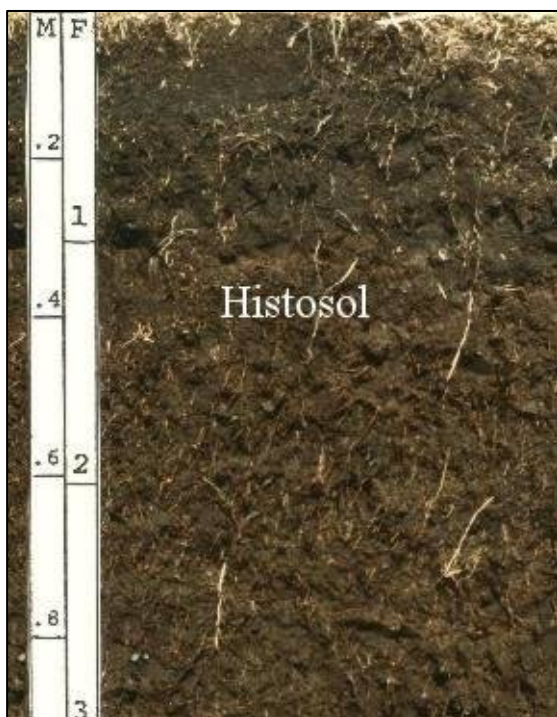
Figure 3-1. Indicator A1 (Histosol). In this example, muck (sapric soil material) is greater than 3 ft (0.9 m) thick.
