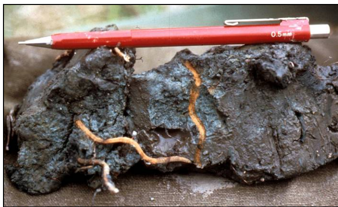
Figure 4-20. Iron oxide plaque (orange coating) on a living root (center left). Iron also coats the channel or pore from which the root was removed (center).
