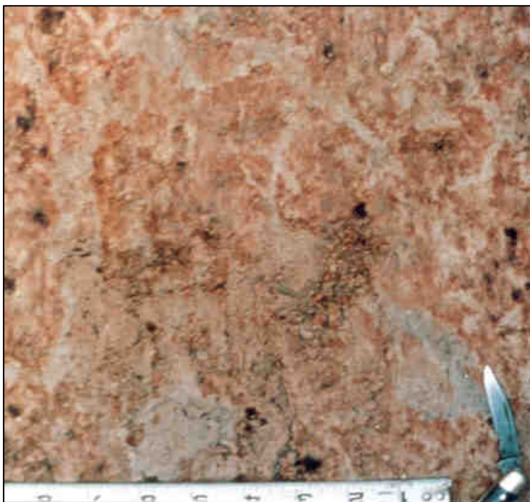
Figure 3-26. Iron-manganese masses (black spots) in a 40 percent depleted matrix. Scale is in inches.
