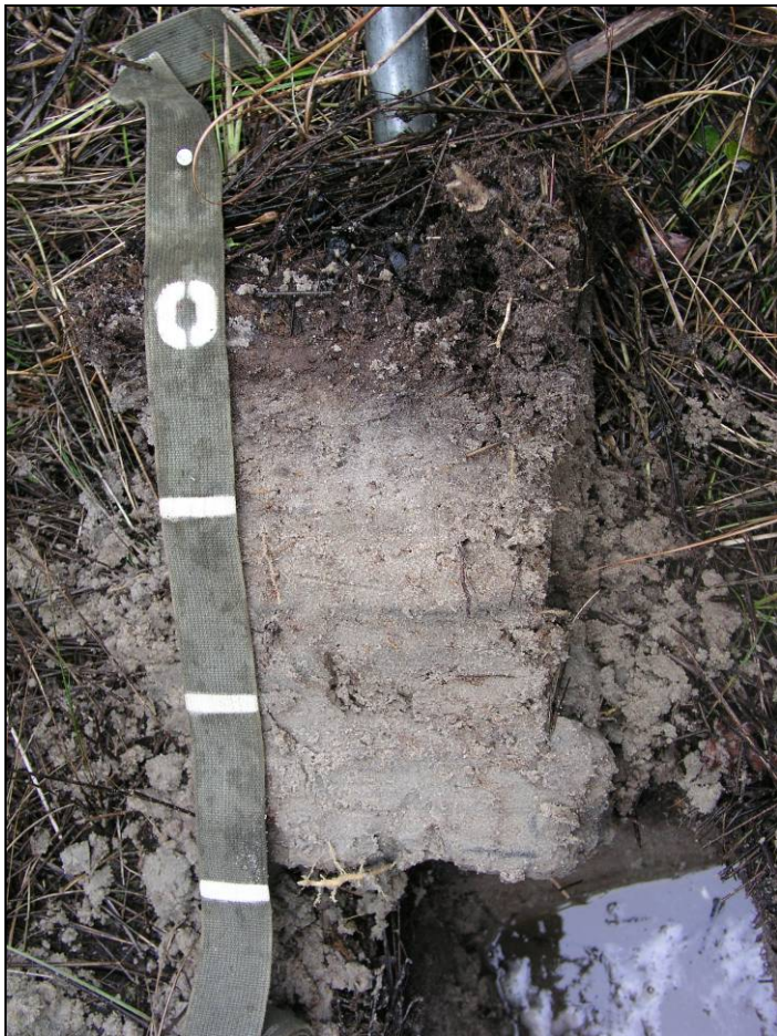
Figure 5-6. Soil with a mucky-peat surface over sand. Increments on tape are 4 in. (10 cm).
