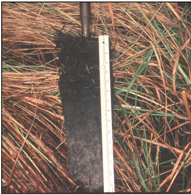
Figure 16. The mucky modified sandy layer is approximately 3 in. (7.5 cm) thick. Scale in inches on the right side of ruler.
