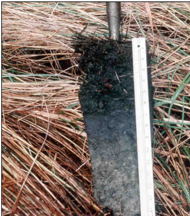
Figure 20. This sandy soil has a dark surface approximately 6 in. (15 cm) thick. Scale in inches on right.
