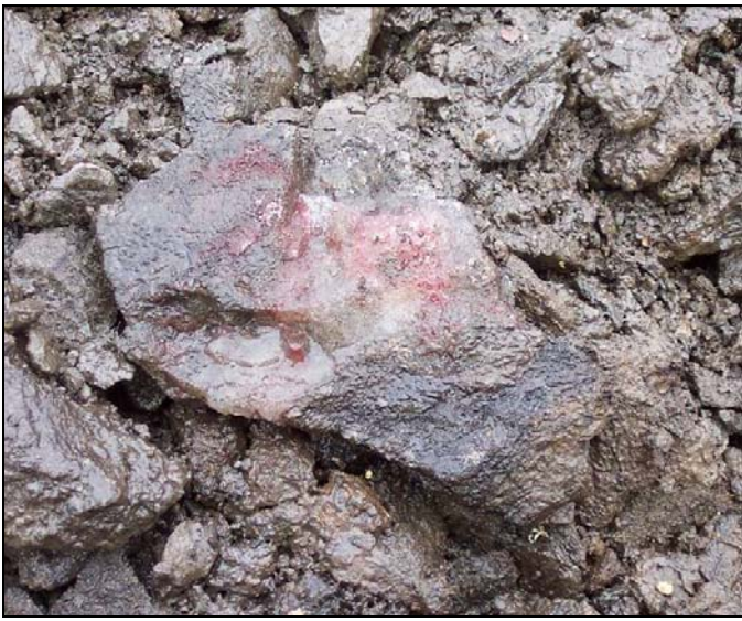
Figure 53. When alpha, alpha-dipyridyl dye is applied to a soil containing reduced iron, a positive reaction is indicated by a pink or red coloration to the treated area.
