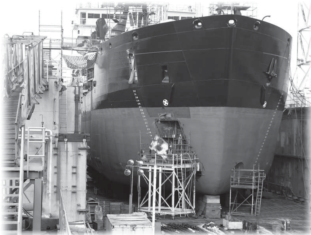
Workers transfer new equipment through the dredge Essayons ' bow. The dredge, which began service in 1983, is undergoing an extensive upgrade of its engines and systems, which will take three years to complete between dredging work periods.
