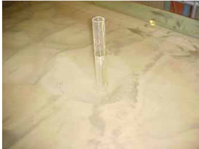
Figure A11. Final photo of scour hole; flow from right to left.
