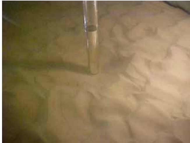
Figure B40. Final photo of scour hole; flow from right to left.
