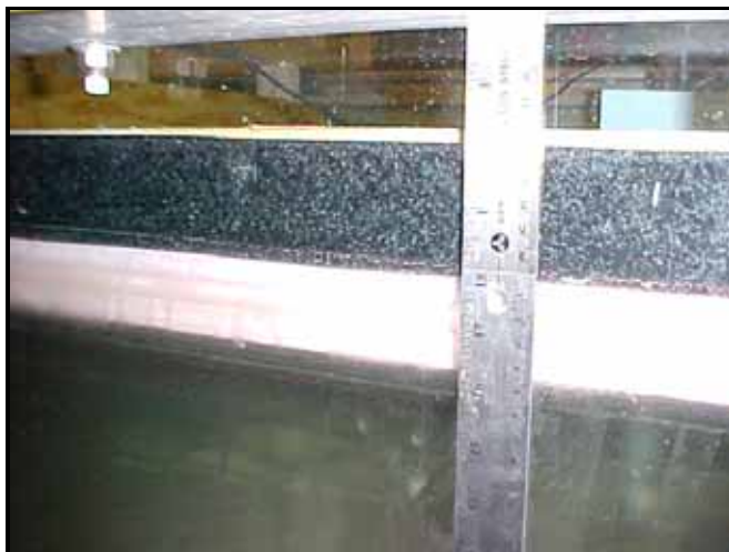
Figure 16. Foam seals along the sides of the simulated ice cover.
