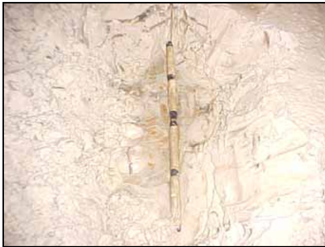
Figure 30. Copper tubing installed in the floor of the flume.
