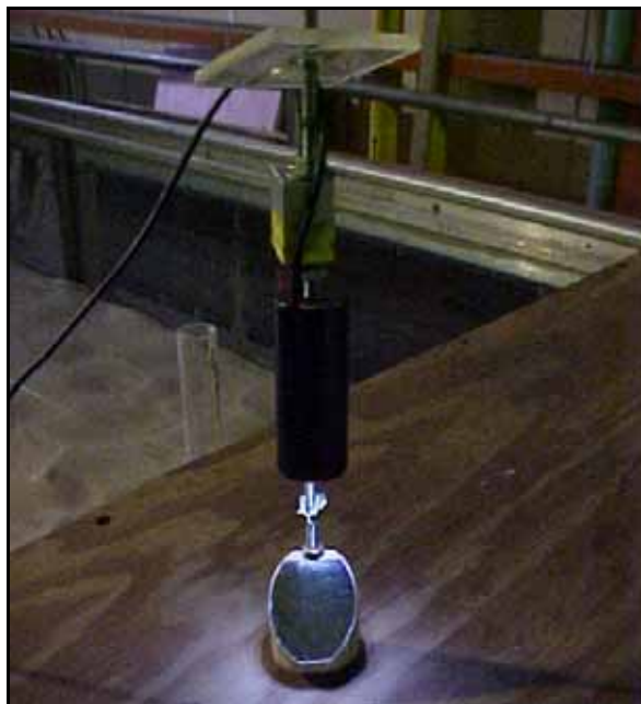
Figure 18. Camera-mirror assembly to measure scour depth at the pier.
