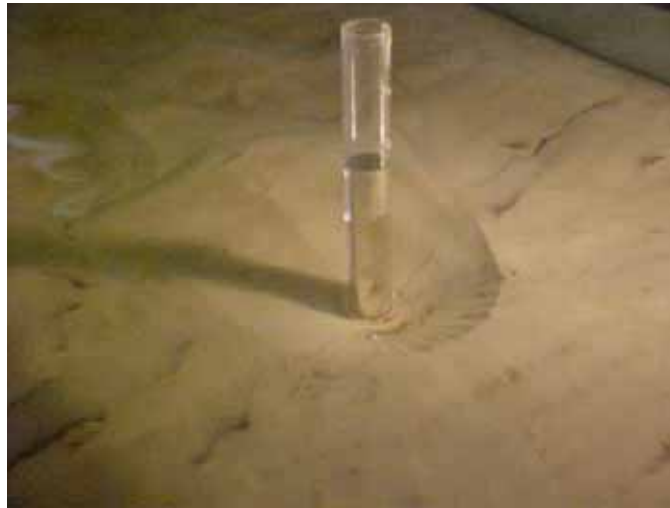
Figure C33. Final photo of scour hole; flow from right to left.
