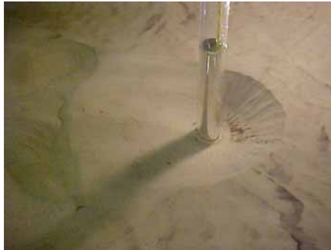
Figure C26. Final photo of scour hole; flow from right to left.
