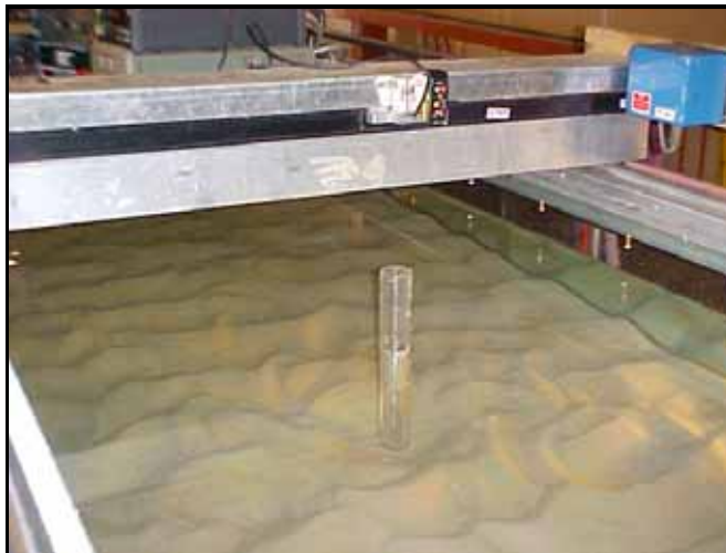
Figure 36. Final scour hole profiling for test XR2.
