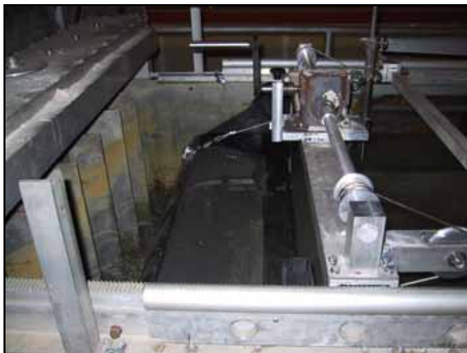
Figure 6. Adjustable weir used to control the water surface level in the flume.
