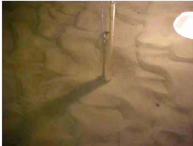
Figure C19. Final photo of scour hole; flow from right to left.
