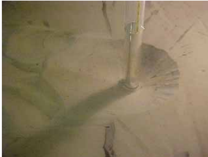
Figure A39. Final photo of scour hole; flow from right to left.
