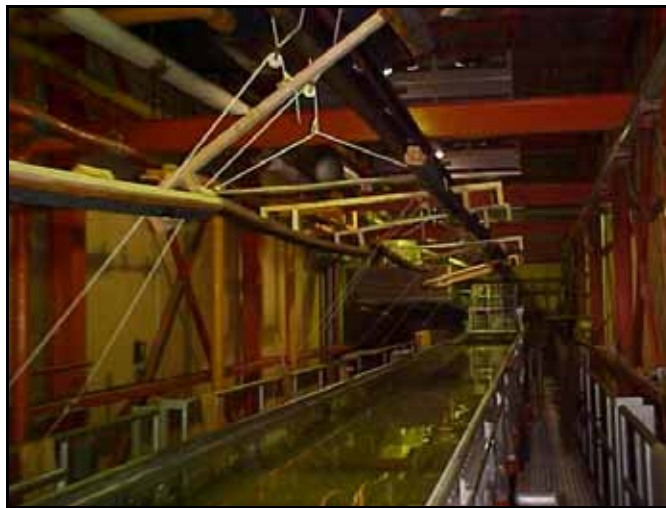
Figure 15. Raised ice restraint system.
