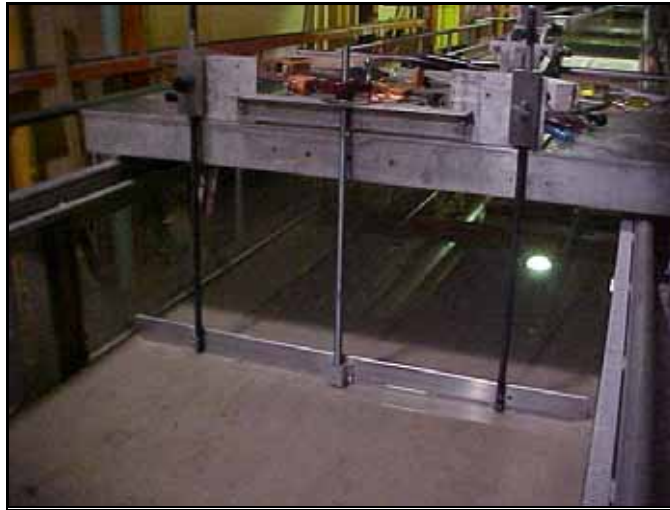
Figure 34. Bed leveling device attached to a movable carriage.
