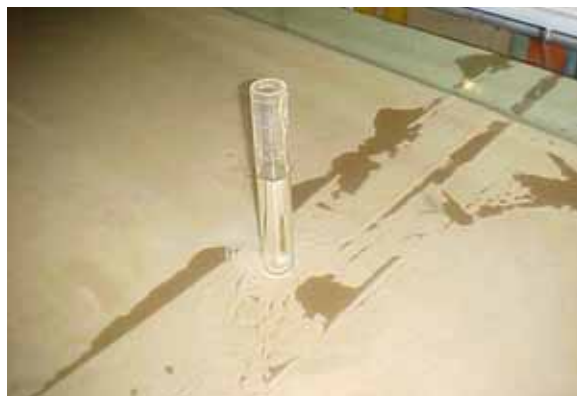
Figure A4. Final photo of scour hole; flow from right to left.
