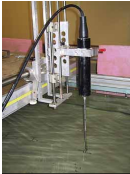
a. ADV mounted over flume.
