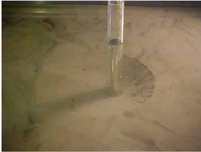
Figure B5. Final photo of scour hole; flow from right to left.
