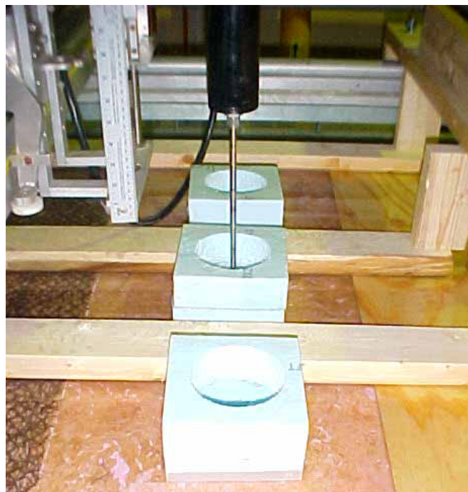
Figure 27. Velocity profiling with the fixed ice cover. The Styrofoam wells prevented water from flowing up onto the surface of the ice cover.
