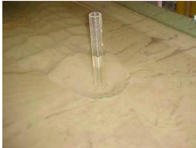
Figure A18. Final photo of scour hole; flow from right to left.
