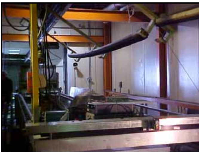
Figure 17. Raised ice restraint system allowed for the instrument carriage to be positioned.
