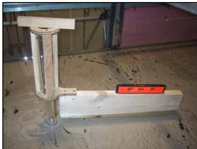
Figure 33. Device used to level the area around the pier.
