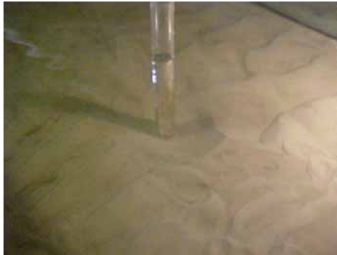
Figure C12. Final photo of scour hole; flow from right to left.
