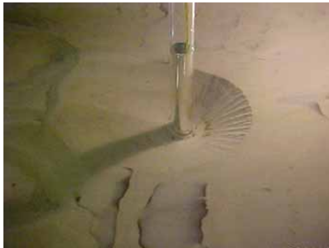
Figure C40. Final photo of scour hole; flow from right to left.
