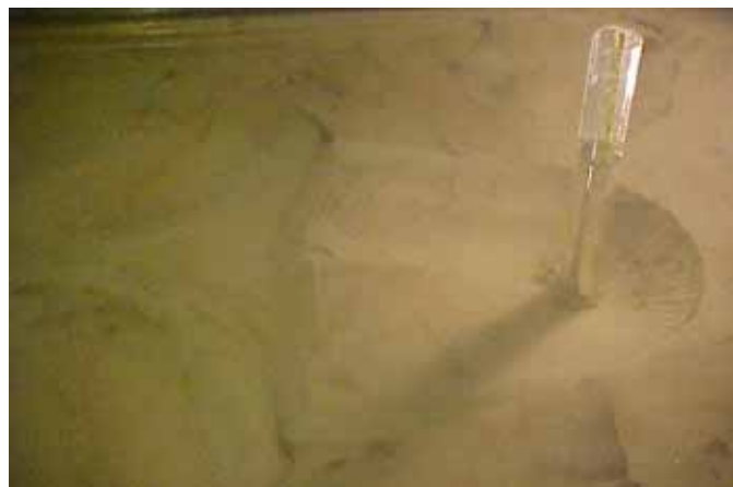
Figure B12. Final photo of scour hole; flow from right to left.
