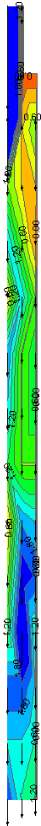
Figure 18. Vertical velocity profile along centerline of the model Poe Lock Case 2a: Flushing ice from chamber with existing split-bottom lateral F/E system plus ports in lower miter gates.
