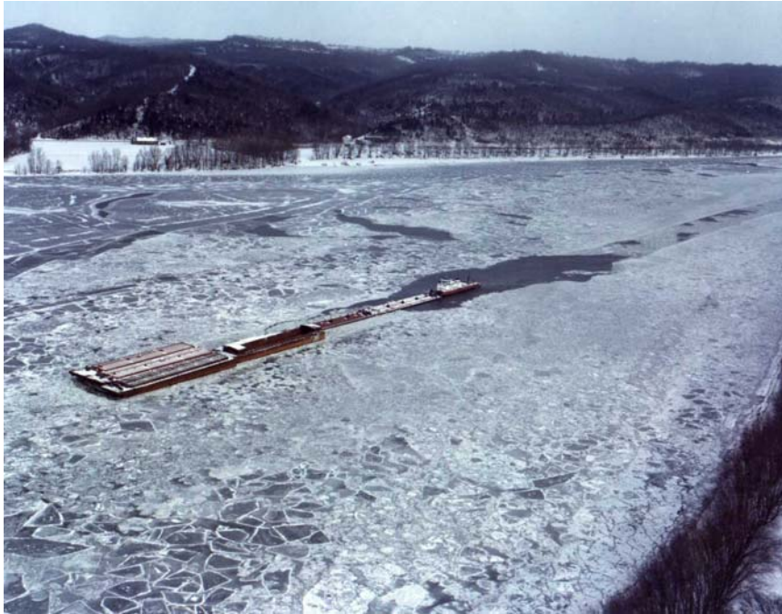
Figure 2. Tow breaking through frozen brash ice on the Ohio River.
