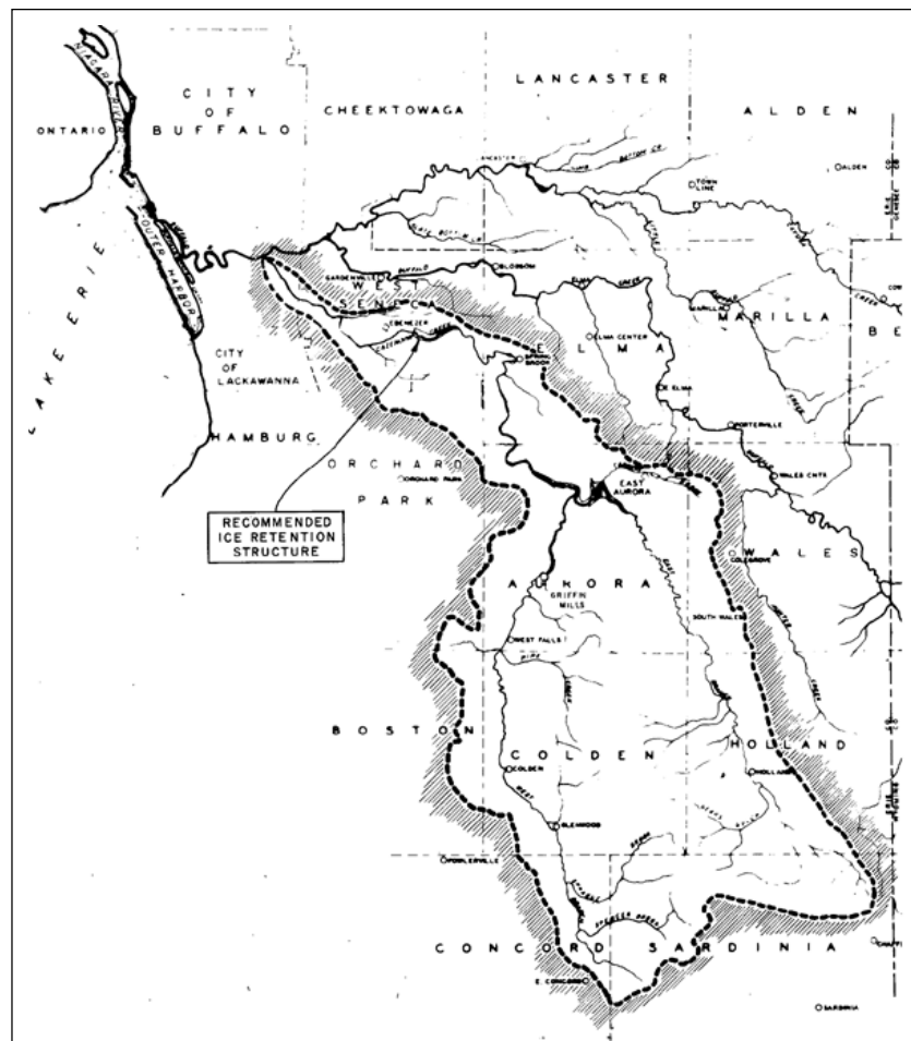
Figure 1. Cazenovia Creek drainage basin. (From USACE 1975.) The new cylindrical-pier ICS would be located at the same site originally proposed for a weir-with-piers ICS or “ice retention structure” (USACE 1986a, 1986b).
