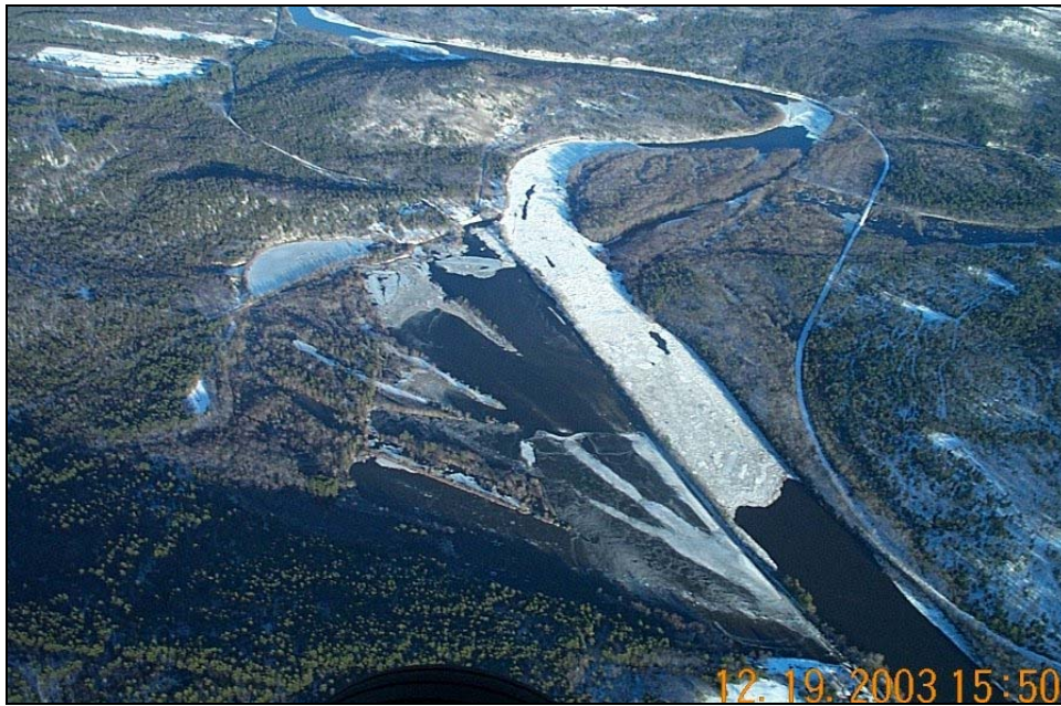
Figure 5. 2003 ice jam on the Androscoggin River in Maine causing overbank flooding and sediment deposition.
