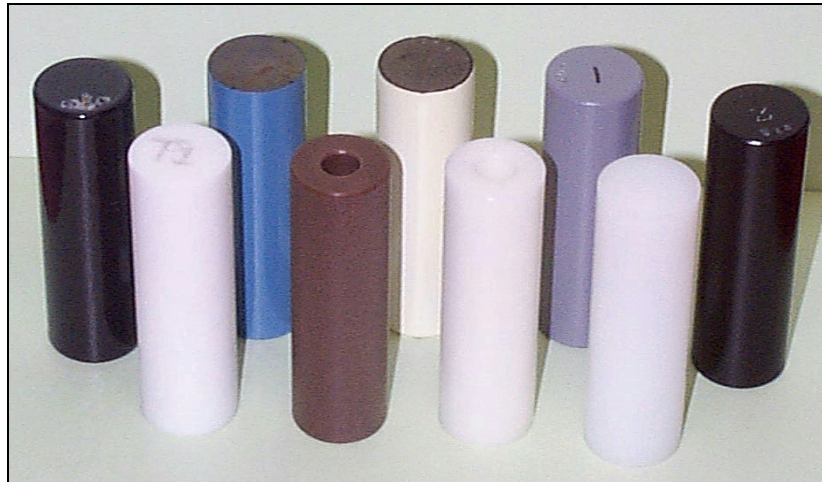
Figure 3. Several thermoplastic (front) and coated-steel sample piles (rear).
