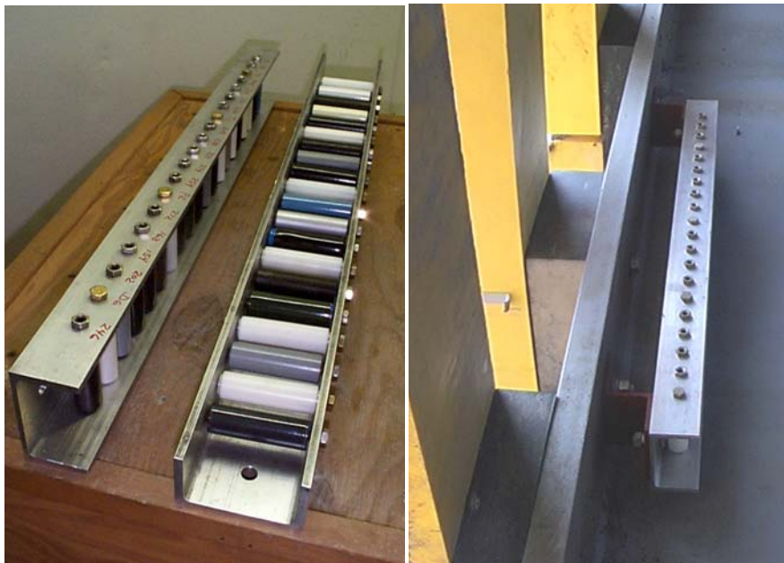
b. (Left) Two sample racks, each with 20 piles randomly ordered for field testing. (Right) Sample rack in place behind gate rub rails.
