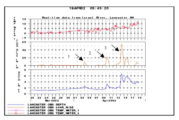
Figure 4. Lancaster Web page interface, showing three events. The first event did not exceed alarm thresholds and did not result in flooding. The second and third events did trigger alarms.
