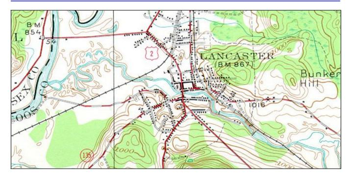
Figure 3. Contour map of Lancaster, New Hampshire (USGS 1935.) Two former dams and their impoundments are shown. The other two former dams were located just upstream and downstream of the Main Street (Route 2) Bridge. Damaging ice jams now form at the upstream end of the backwater from the Connecticut River, near the railroad crossing.
