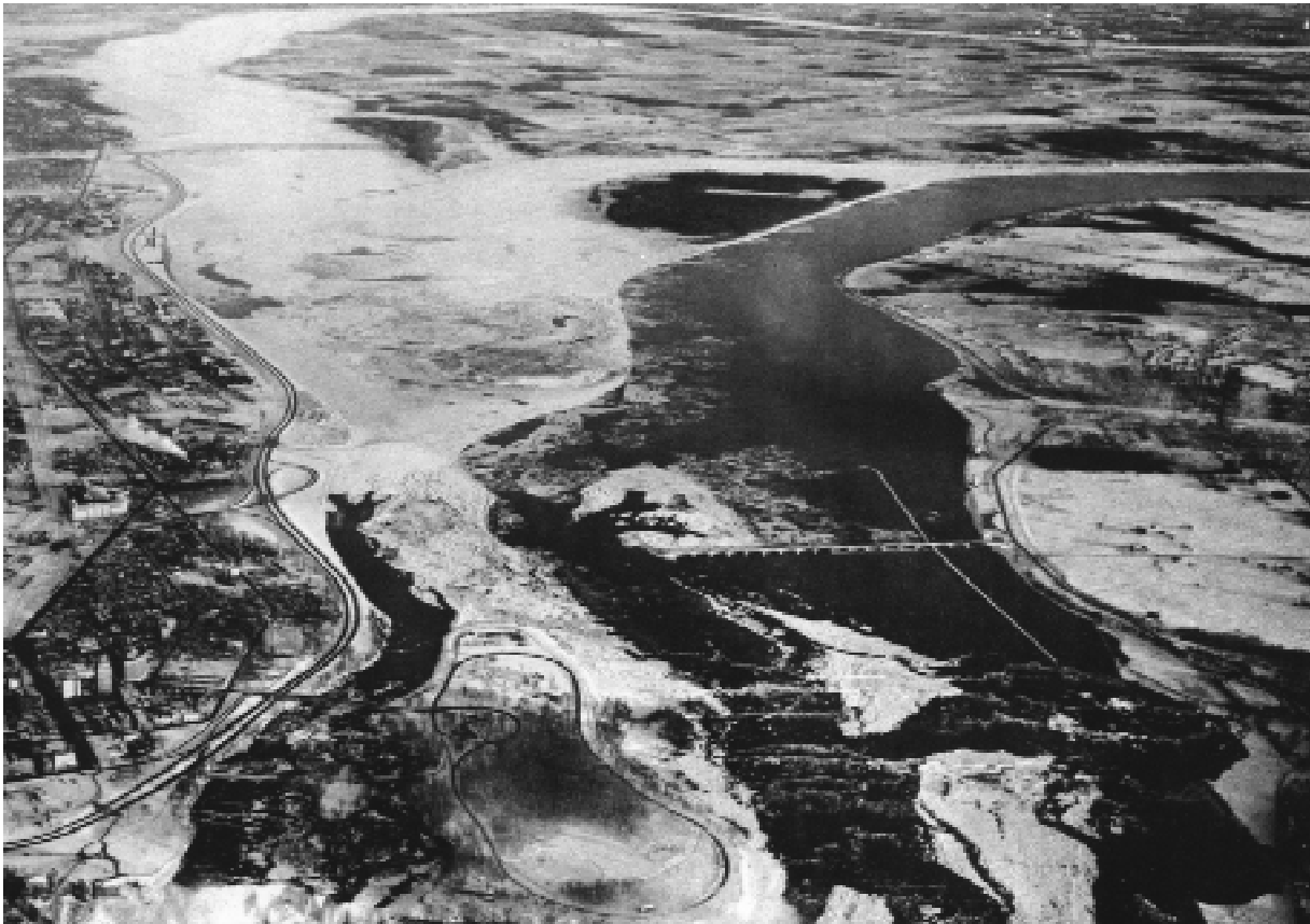
Figure 6. Ice jam at the intakes of the NYPA Niagara Falls Power Project on the Upper Niagara River. (Photo courtesy of P.A.S.N.Y.)
