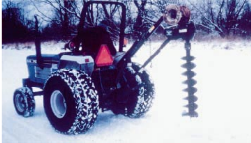
a. Posthole digger mounted on the back of a tractor.
