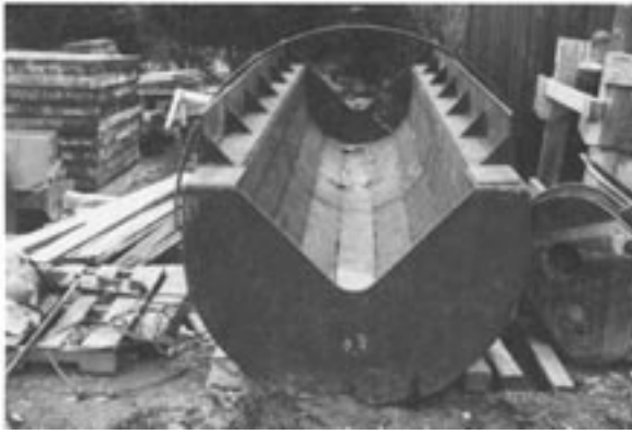
Figure 9. Inner surface of the load beam.
