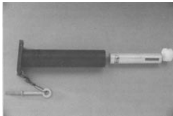
Figure 11. Assembly of the instrumented fish, including an eyebolt, a swivel, a polyethylene housing, a transmitter and an end cap.
