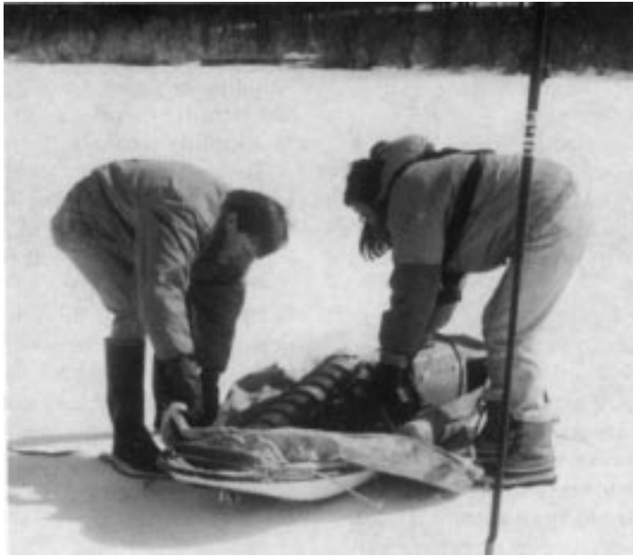
a. Sleds can be used to haul equipment and provide emergency flotation.
