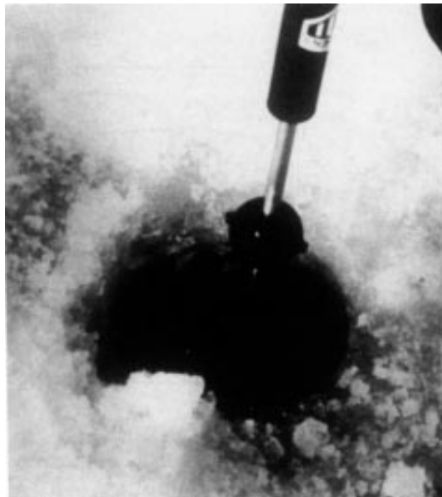
b. The sensor has no moving parts to freeze when removed from the water.
