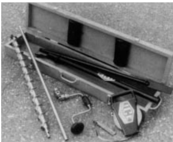
a. Standard CRREL ice thickness measuring kit. From left, auger with carbide-tipped bit, extension rod, bit brace, and ice thickness measuring device. In the box is a two-part iron bar (hollow top, solid bottom) that can be screwed together for field work and disassembled for transport.
