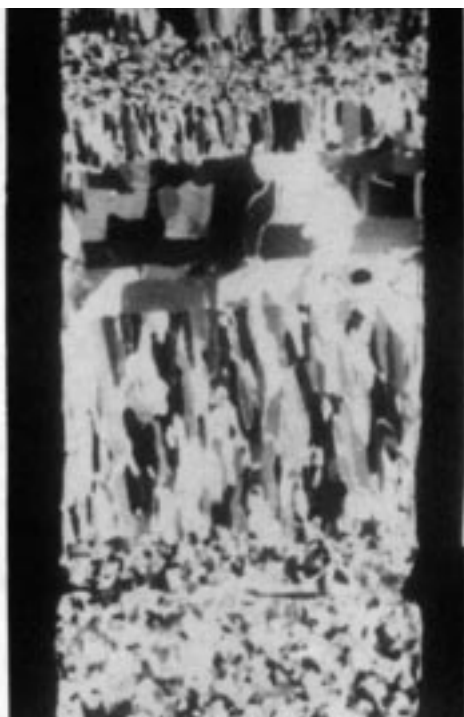
Figure 16. Thin section of an ice cover. The long slender crystals in the center represent ice growth due to heat transfer; the more chaotic ice in the lower section is frazil ice. The upper portion contains snow ice, frozen rainwater, and both frazil and thermally grown ice (Israel River, N.H.).
