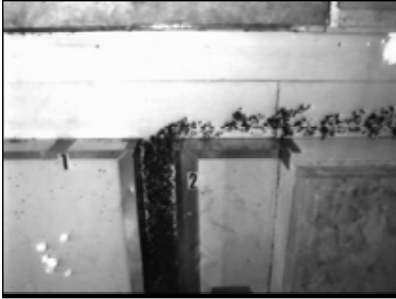
Figure 24. Ice in confluence: Q_2/Q_1 = 2/3 , \alpha = 90^\circ , and b_1/b_2 = 3 .
