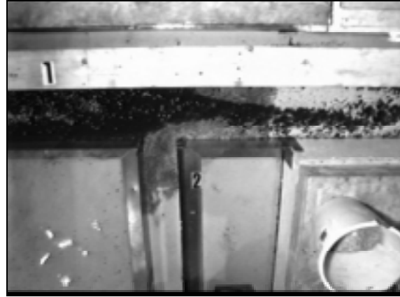
Figure 22. Ice in confluence: Q_2/Q_1 = 3 , \alpha = 90^\circ , and b_1/b_2 = 1.5 , bathymetry modeled.
