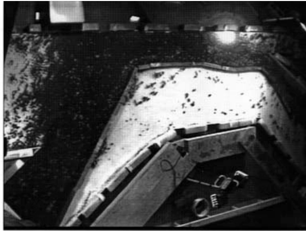
Figure 47. Ice congestion for the confluence with border ice (without bendway weirs).
