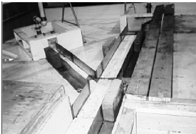
Figure 11. View of the jam process model configured for a 45° confluence.
