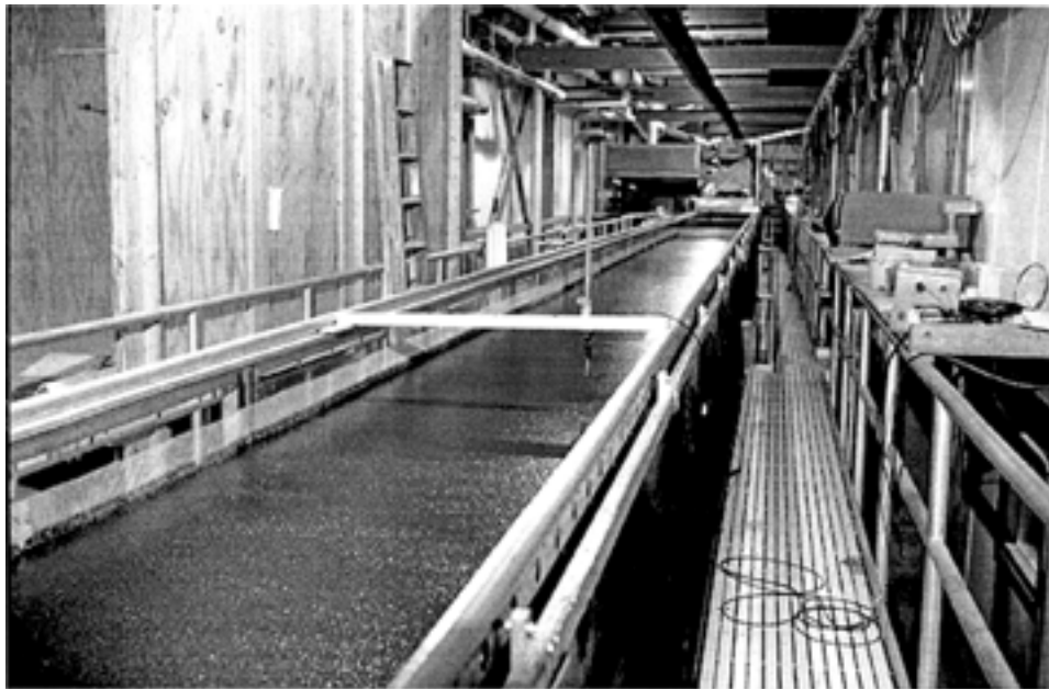
Figure 15. CRREL refrigerated, tiltable flume.
