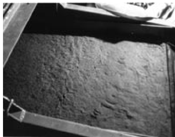
Figure 29. Sand bed of model bank deformed by ice action after test 8.
