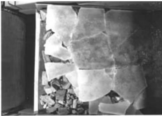
Figure 18. Ice sheet after it is broken and pushed up the riprap bank.
