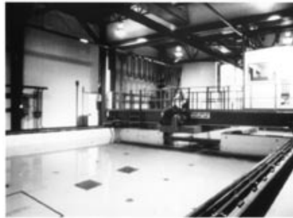
Figure 11 Refrigerated test basin in the Ice Engineering Facility.
