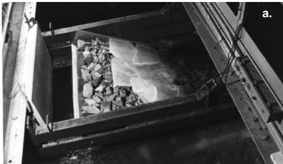
Figure 18. Ice sheet after it is broken and pushed up the riprap bank.
