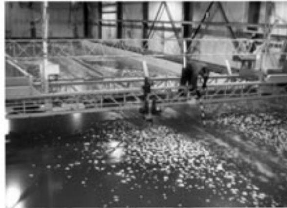
Figure 15. Cutting of slots in the model ice sheet prior to each test.
