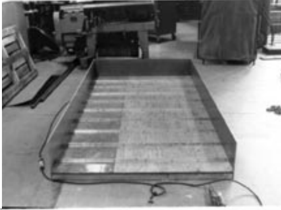
Figure 6. Aluminum box used for model riprap bank.
