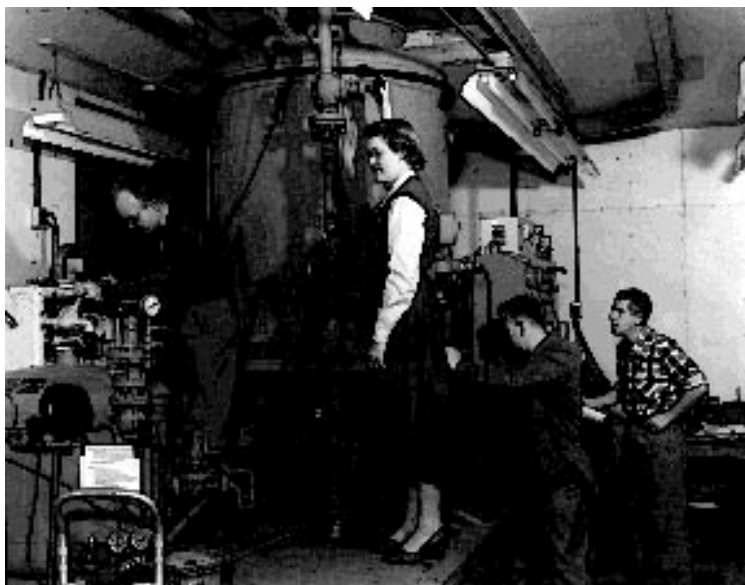
Tom Noggle, Jean Redman, Ralph Coltman, and Tom Blewitt (l to r) are shown preparing refrigeration equipment for in-pile low-temperature experiments at the Oak Ridge Graphite Reactor.
