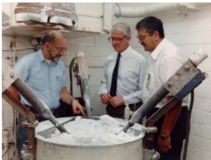
Marvin Abraham (left) and Lynn Boatner (center) discuss the submerged arc-fusion growth of MgO single crystals with Commercial Crystal Laboratories (CCL) President Michael Urbanik (right). CCL was a partner in a CRADA with ORNL to improve the size and quality of MgO single crystals.
