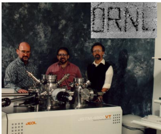
David Zehner, Joe Carpinelli, and Ward Plummer (l to r) examine the JEOL STM used to write the ORNL logo shown in the inset. At this scale ( 400 \times 800 \text{ \AA}^2 ), 15 complete copies of the Encyclopaedia Britannica could be written on the head of a pin. The image was provided by Carpinelli, winner of the 1996 Nottingham Prize (Physical Electronics Conference).
