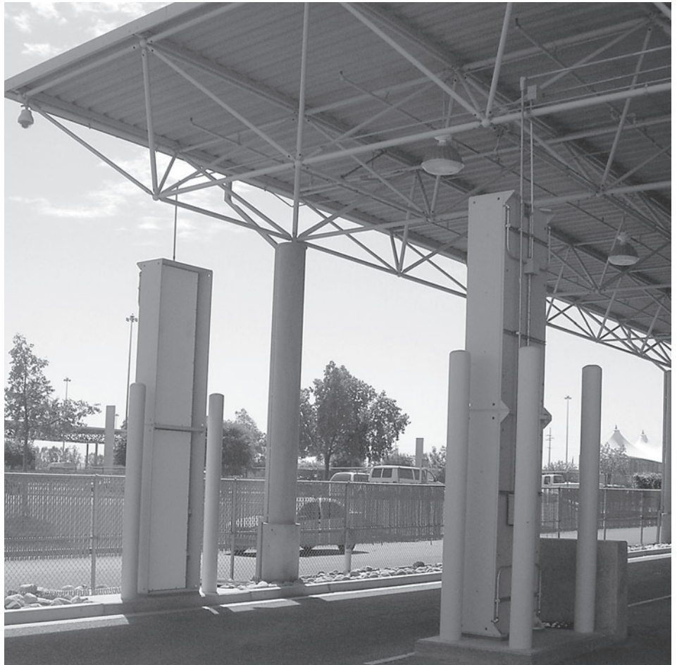
Figure 4: Truck-Sized Portal Monitor in the Inspection Area at a Port of Entry on the Southern Border
