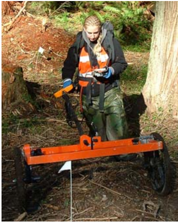
A technician uses the EM-61 to refine an anomaly for investigation. (Photo by Wayne Martrildonno)
