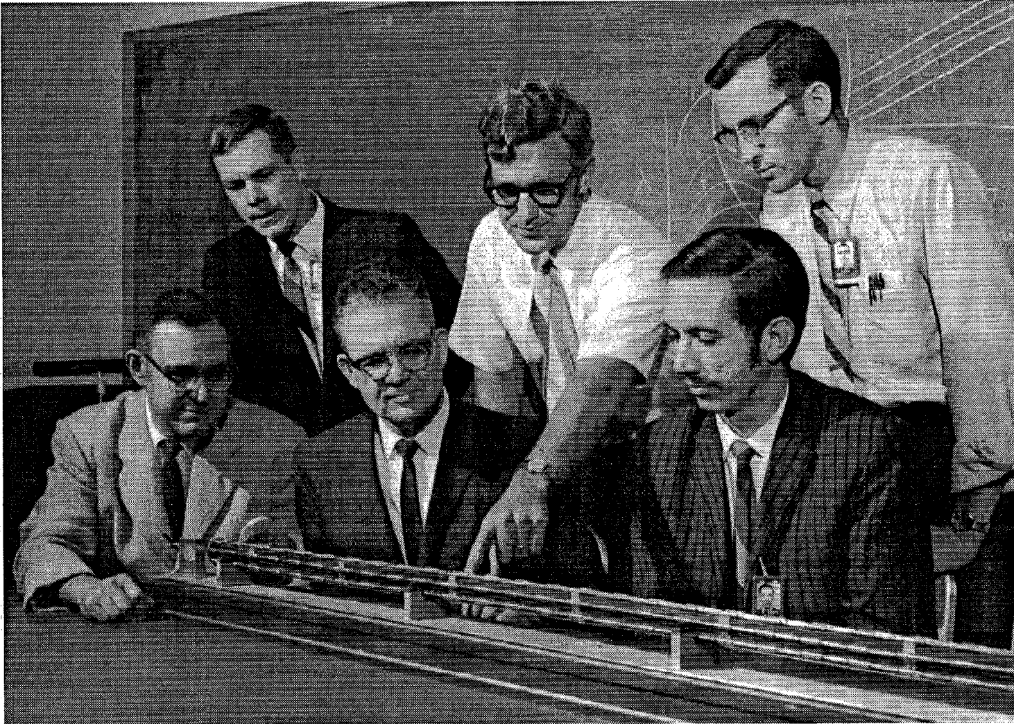
Fig. 8. In-reactor surveillance irradiation experiment to be placed in the Molten Salt Reactor Experiment. The purpose was to determine the compatibility of Hastelloy N and graphite under irradiation and molten salt corrosion conditions. (left to right, Arnold P. Litman, Charles E. Sessions, W. Howard Cook, C. Ray Kennedy, John W. Roger, and Ron L. Beatty).
