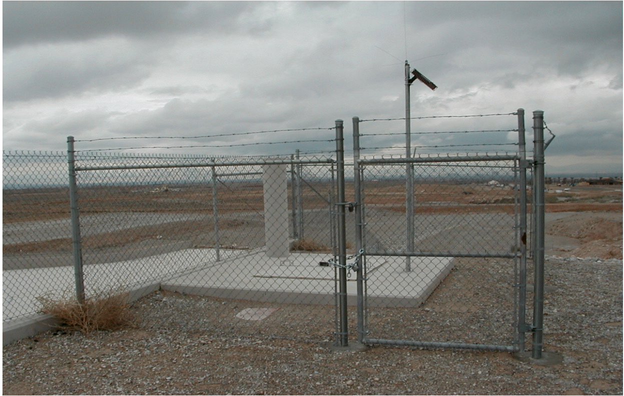
Photo 4. Red Rock Detention Basin . Instrumentation vault and precipitation gage (cylindrical structure).
