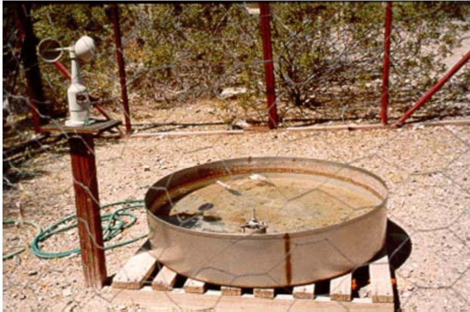
Photo 5-01. Evaporation pan at Alamo Dam and Lake.
