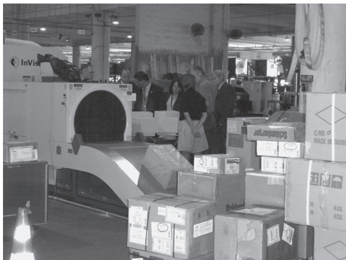
Figure 4: Air Cargo Being Loaded and Inspected Using an Explosive Detection System
