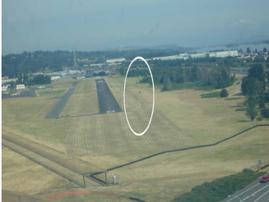
Figure B-7. Flight Evaluation Left of Baffled Line—VASI Signal Visible
