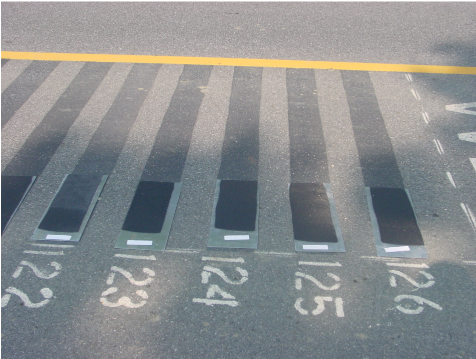
FIGURE 2. BLACK PAINT WITH Q-PANELS
