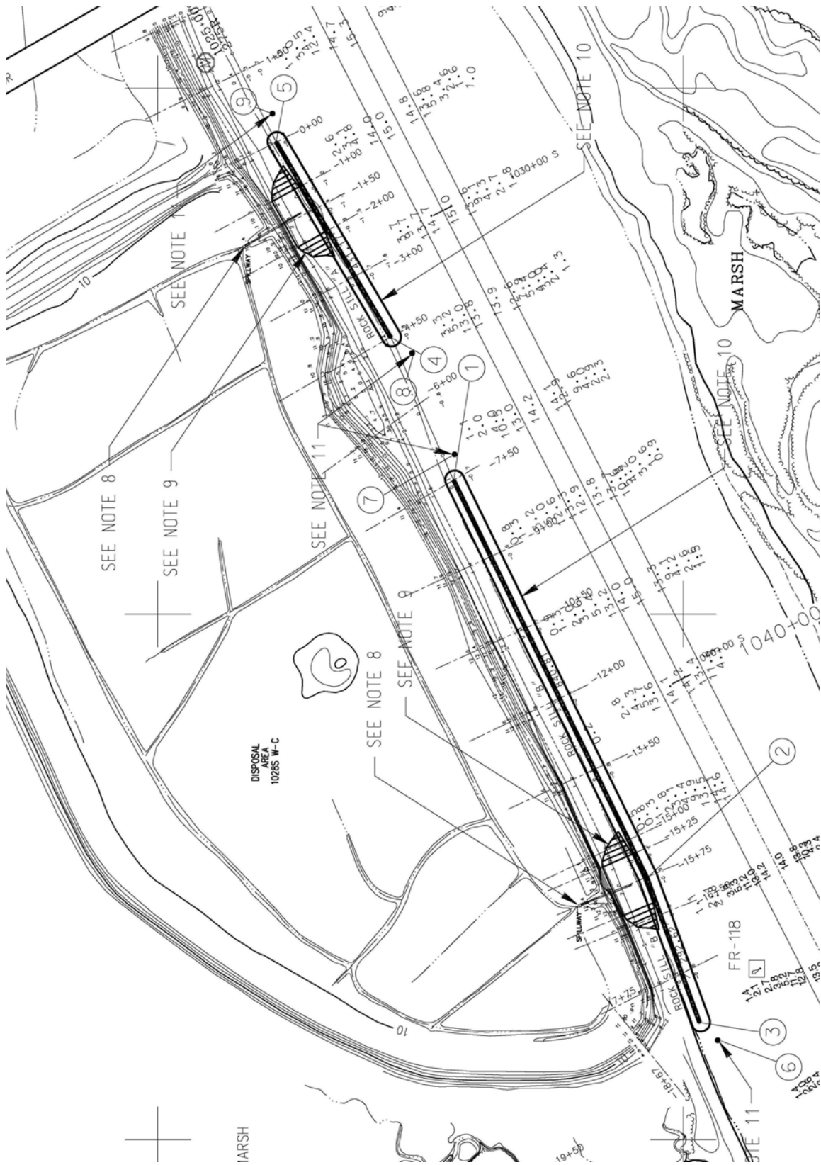
FIGURE 7a – Drain Pipe Locations (Plain View)
