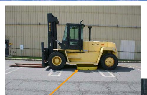
Large drip pan is actually a four drum storage spill container
