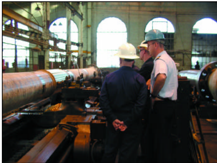
Maintenance and Logistics Command Pacific (MLCPAC) Type Desk, LT Pat Murphy, and Engineer Officer, LT Chad Jacoby, inspect a 378' cutter's propulsion shaft liner while being machined in lathe at San Francisco Drydock.
