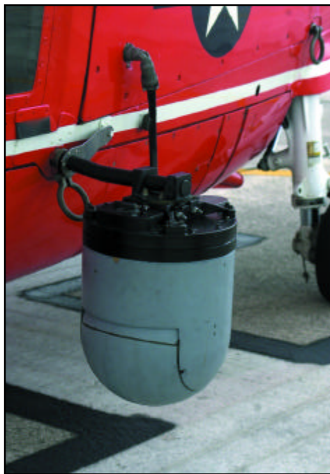
Shown here is a FLIR (Forward Looking Infrared) sensor, one of the Coast Guards many technologies used for search and rescue and law enforcement.
