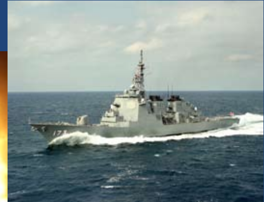
Japanese Destroyer JS Kongo completed Japan's first successful intercept using the Aegis BMD system on December 17, 2007
