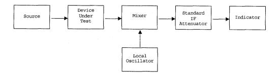
Figure 2. Attenuation measurement by IF substitution.
