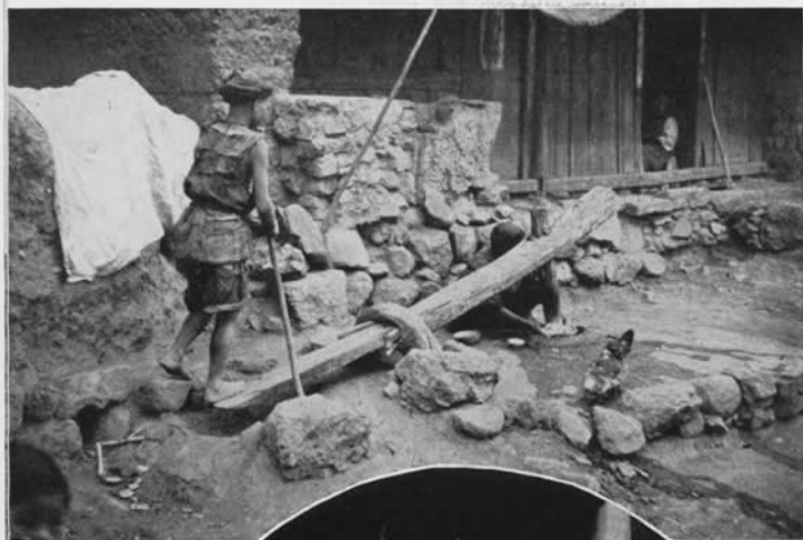
(Below) TWO NATIVES operating a primitive grain mashing machine. Daily life went on in Niu Kai although 150 brigands had been causing trouble in the surrounding hills
