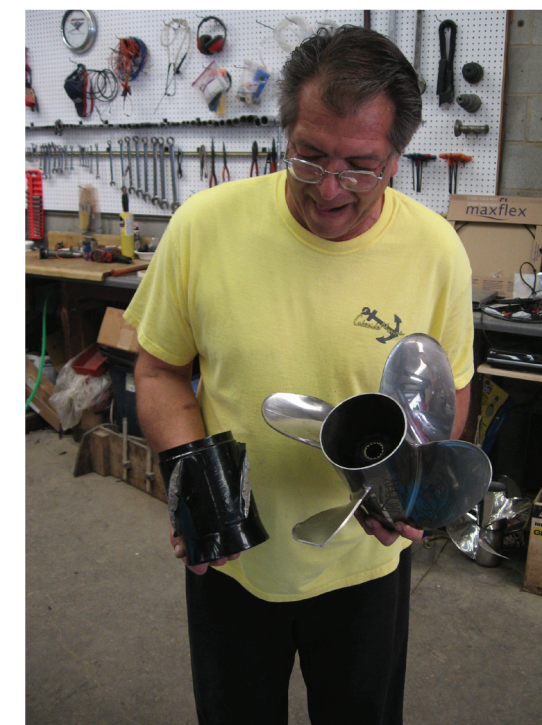
Chuck Chapel, Lakeside Marine, Leah, GA, holds two propellers damaged as a result of a boat collision with a submerged object.
