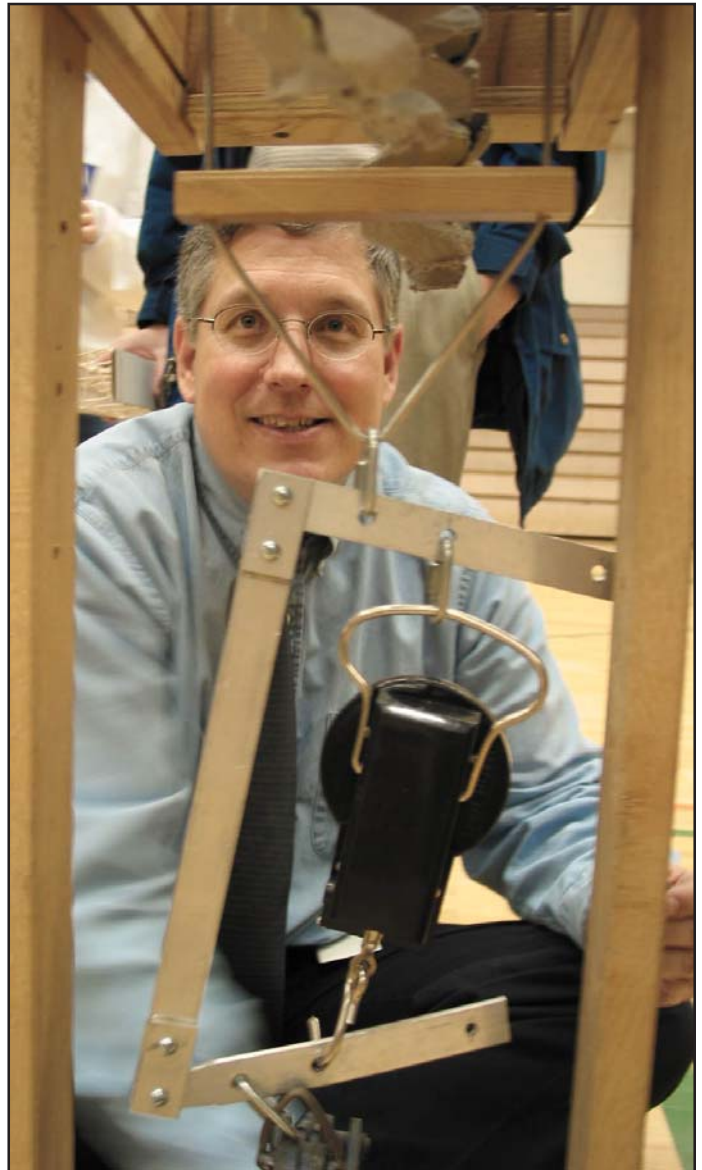
Above, Mark Lindgren, Hydrology and Hydraulics Branch chief, monitors the gauge that measures the amount of force applied to a student's bridge as District engineers test its load capacity. Left, DeSales Catholic School students weigh their bridges prior to testing so they will be able to calculate strength coefficients.
