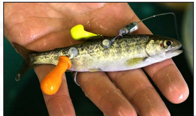
An anesthetized juvenile salmon is fitted with tags to participate in spillway injury tests at Ice Harbor Lock and Dam. Two balloon tags provide a backup in case of inflation failure; a transmitter emits radio waves that can be tracked with a directional receiving antenna; and a unique tiny numerical tag is placed just beneath the skin behind the eye.
