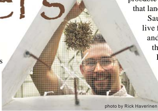
Sauder peers through the bait side of the hair snag trap. Rifle cleaning brushes are arranged to collect hair samples of animals visiting the device.
