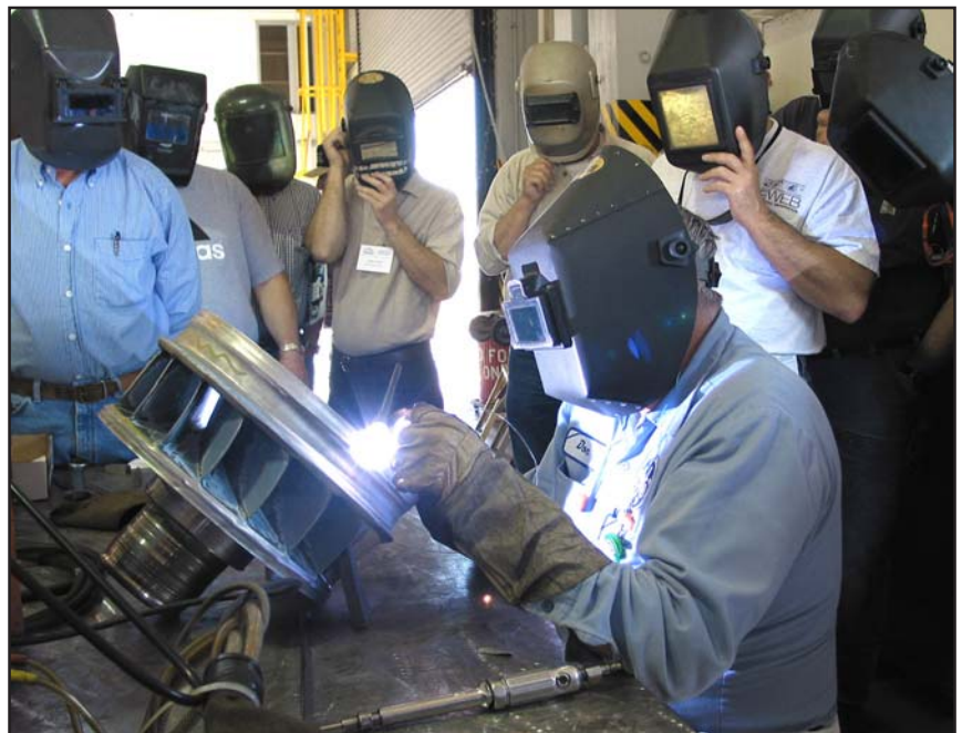
Jeff Phillips, a mechanic at McNary Lock and Dam, shows a workshop attendee from the Eugene Water and Electric Board in Oregon how welders at McNary repair cavitation damage, corrosive-like wear, on the turbine blades and scroll case caused by water flows through the turbine.
