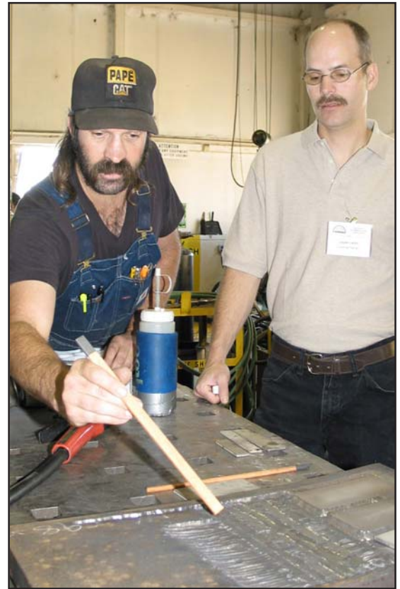
Jeff Phillips, a mechanic at McNary Lock and Dam, shows a workshop attendee from the Eugene Water and Electric Board in Oregon how welders at McNary repair cavitation damage, corrosive-like wear, on the turbine blades and scroll case caused by water flows through the turbine.
